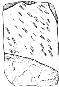
Stone showing typical tooling marks
