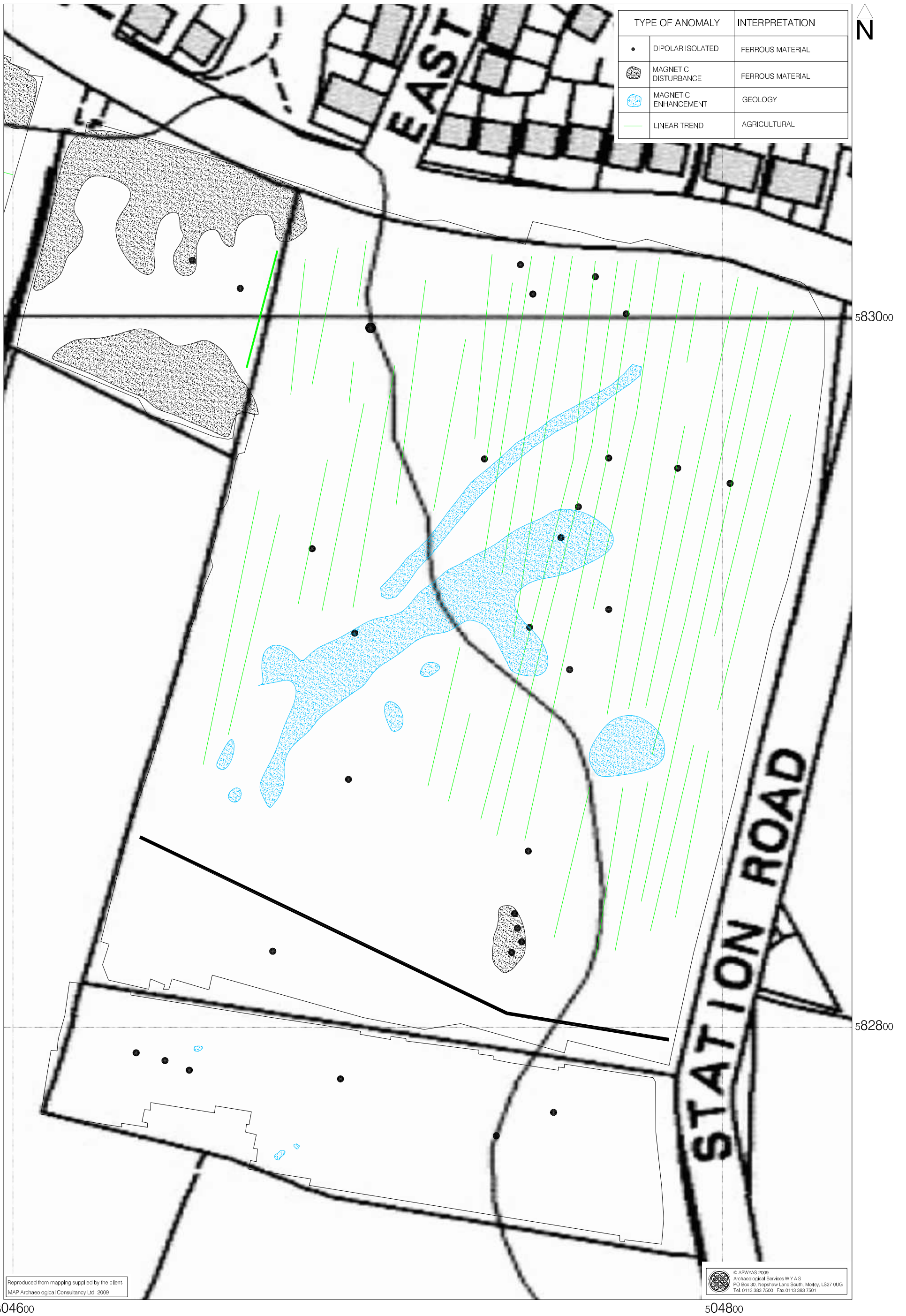
Fig. 8. Interpretation of magnetometer data; Fields 2, 3 and 4 (1:1000 @ A3)
