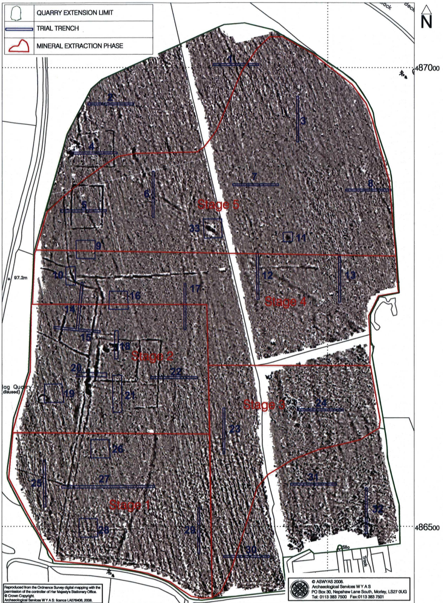
Fig. 2. Grey-scale plot of geophysical survey data and trial trench locations with proposed mineral extraction stages (1-5) (1:2500 @ A4)
