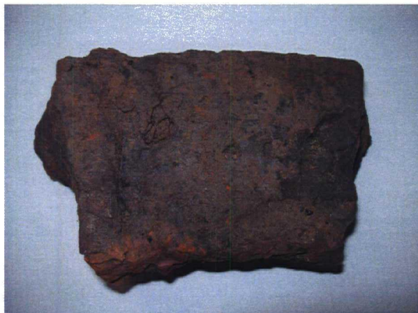
Example of 2 bricks fused together, possibly part of a kiln wall. Context 1009
