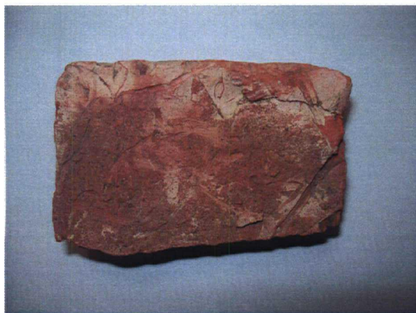
An example of a 'Place' brick. Vegetation impressions indicating that the brick was made on the ground. Context 7009.
