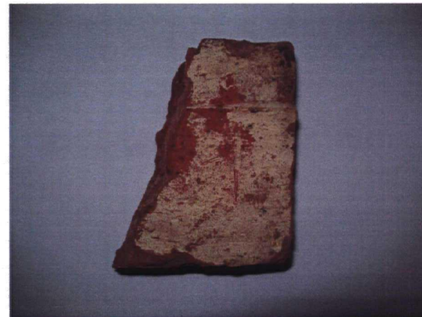
Example of slip on brick, the manufacturers attempt to hide the true colour of the brick. Context 9021
