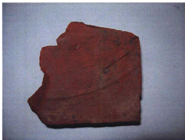
Example of wires used to remove the excess clay from the mould. Context 6002
