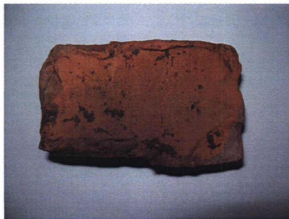
Example of a slop moulded brick. The brick was formed on a sand coated table to prevent sticking. Context 7002
