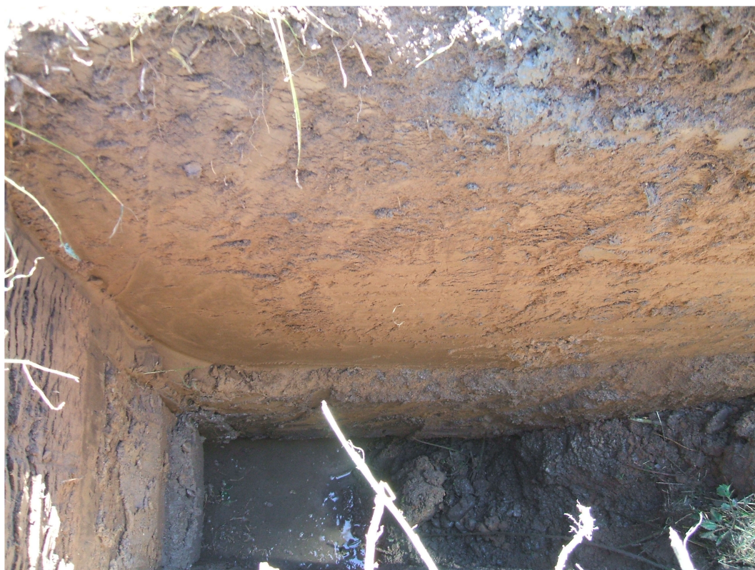
Plate 13 TPSA 119. Organic deposit over gravel in base, clays above
