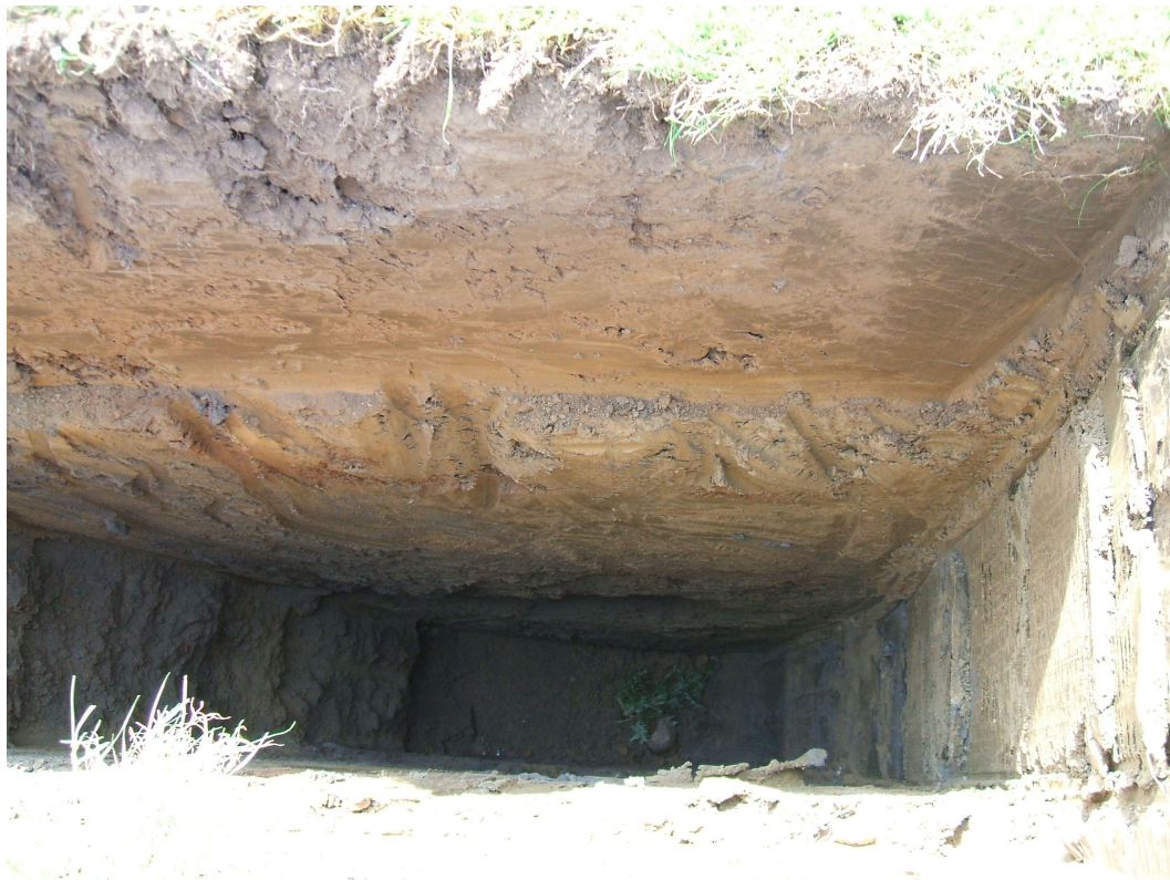
Plate 10 TPSA 111. Clays over shale
