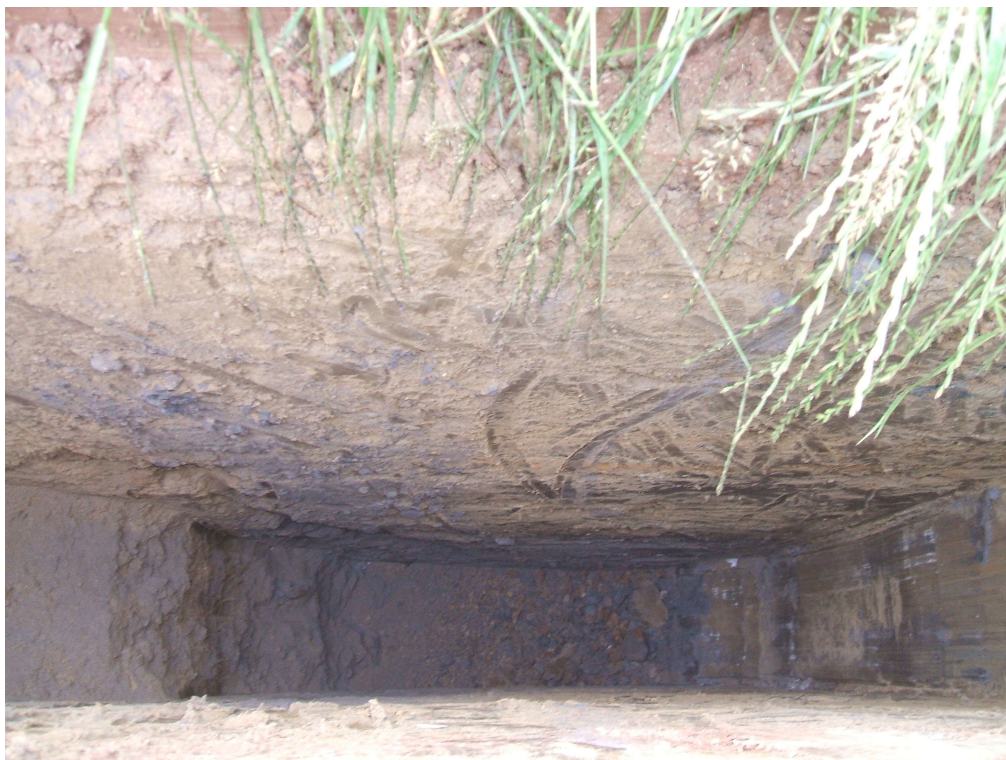
Plate 11 TPSA 113. Mudstone in base, below possible fluvial deposits
