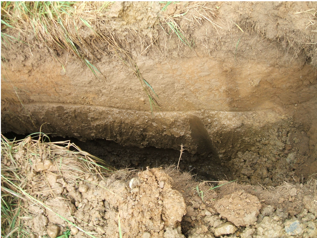
Plate 2 TPTW 002. Clays over gravel
