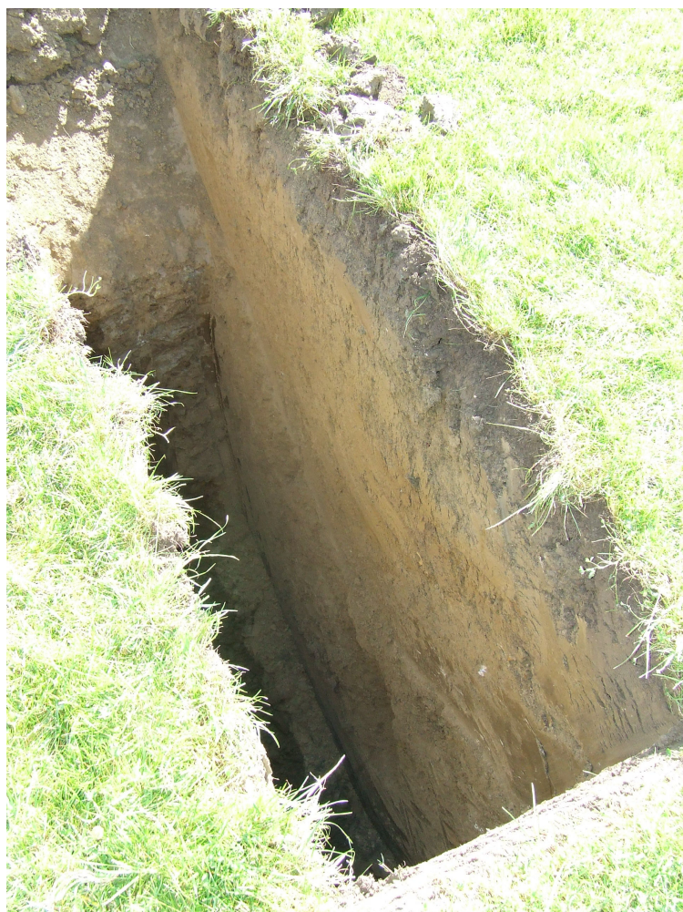
Plate 6 TPSA 009. Clays over silts (alluvium?)
