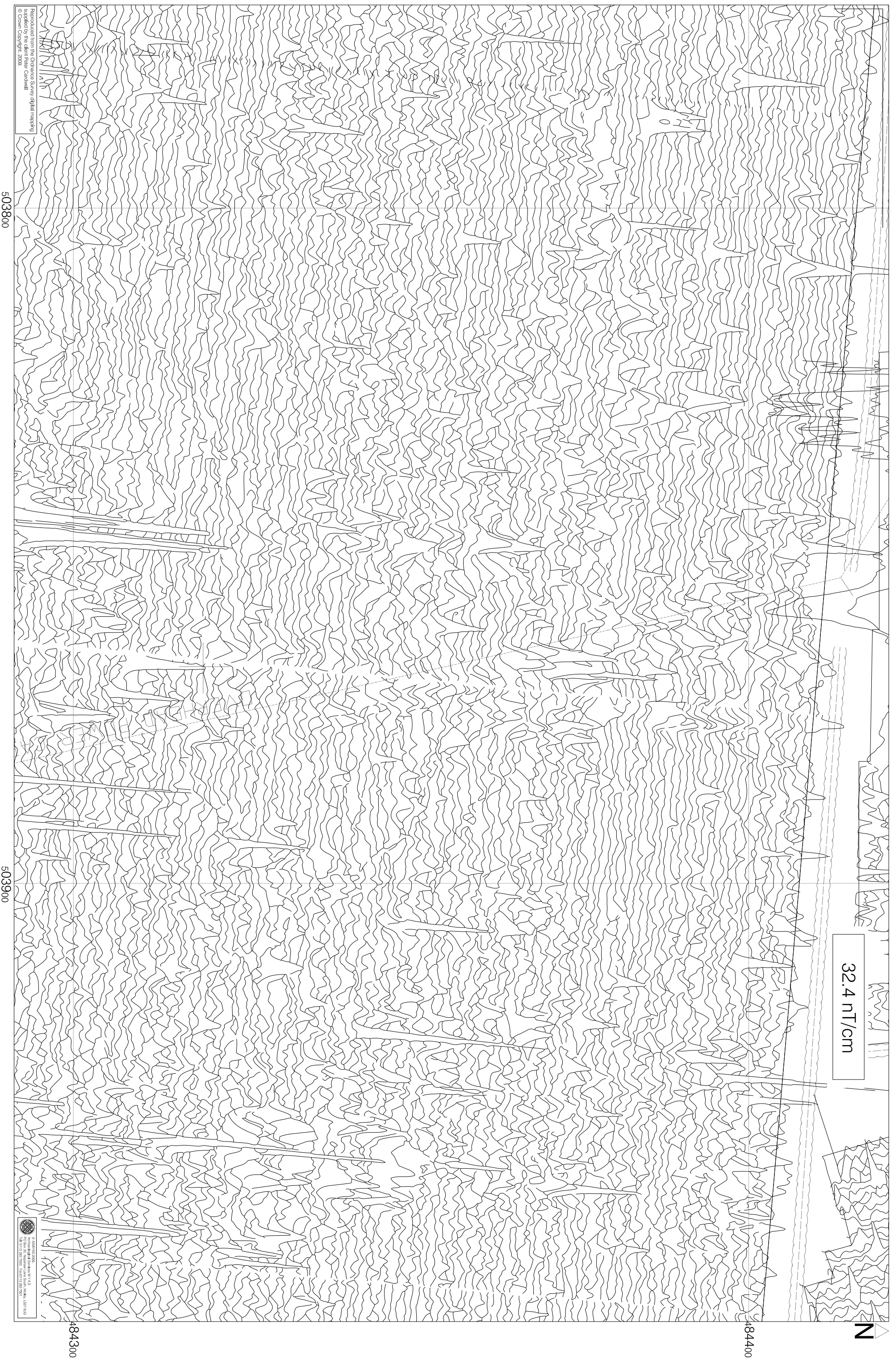
Fig. 51. XY trace plot of unprocessed magnetometer data from Area C, Sector 3 (1:500 @ A3)
