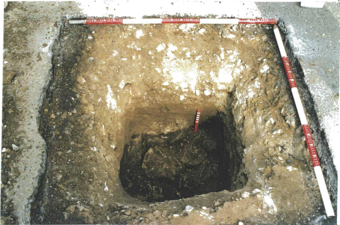
Trial Hole No.3, detailing alluvial deposit and rubble fill.
