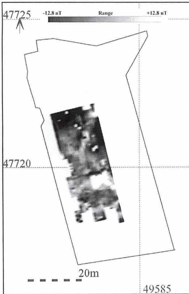
Figure 5 A greyscale image of the magnetic data from the Bartington survey
