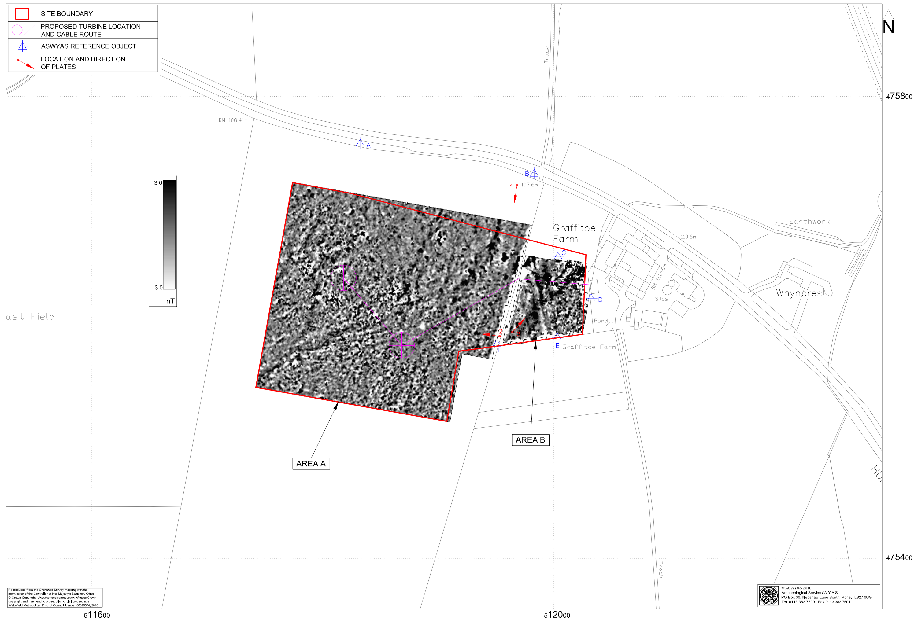
Fig. 2. Site location showing processed geophysical (magnetometer) survey data (1:2000 @ A3)
