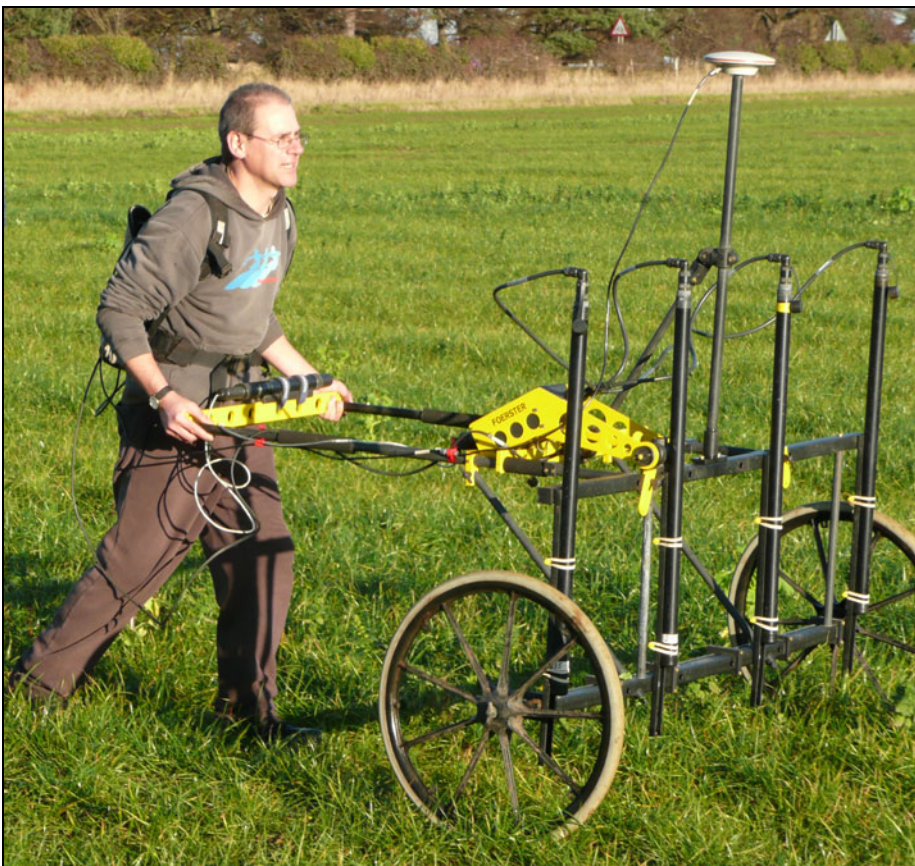
Figure 3 The Foerster gradiometer in operation
