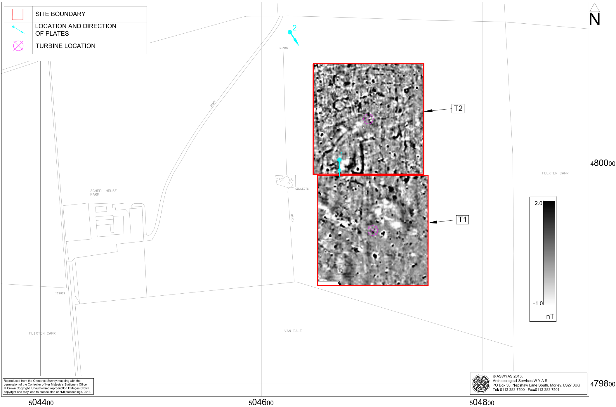
Fig. 2. Survey location showing greyscale magnetometer data and proposed turbine sites (1:2000 @ A4)
