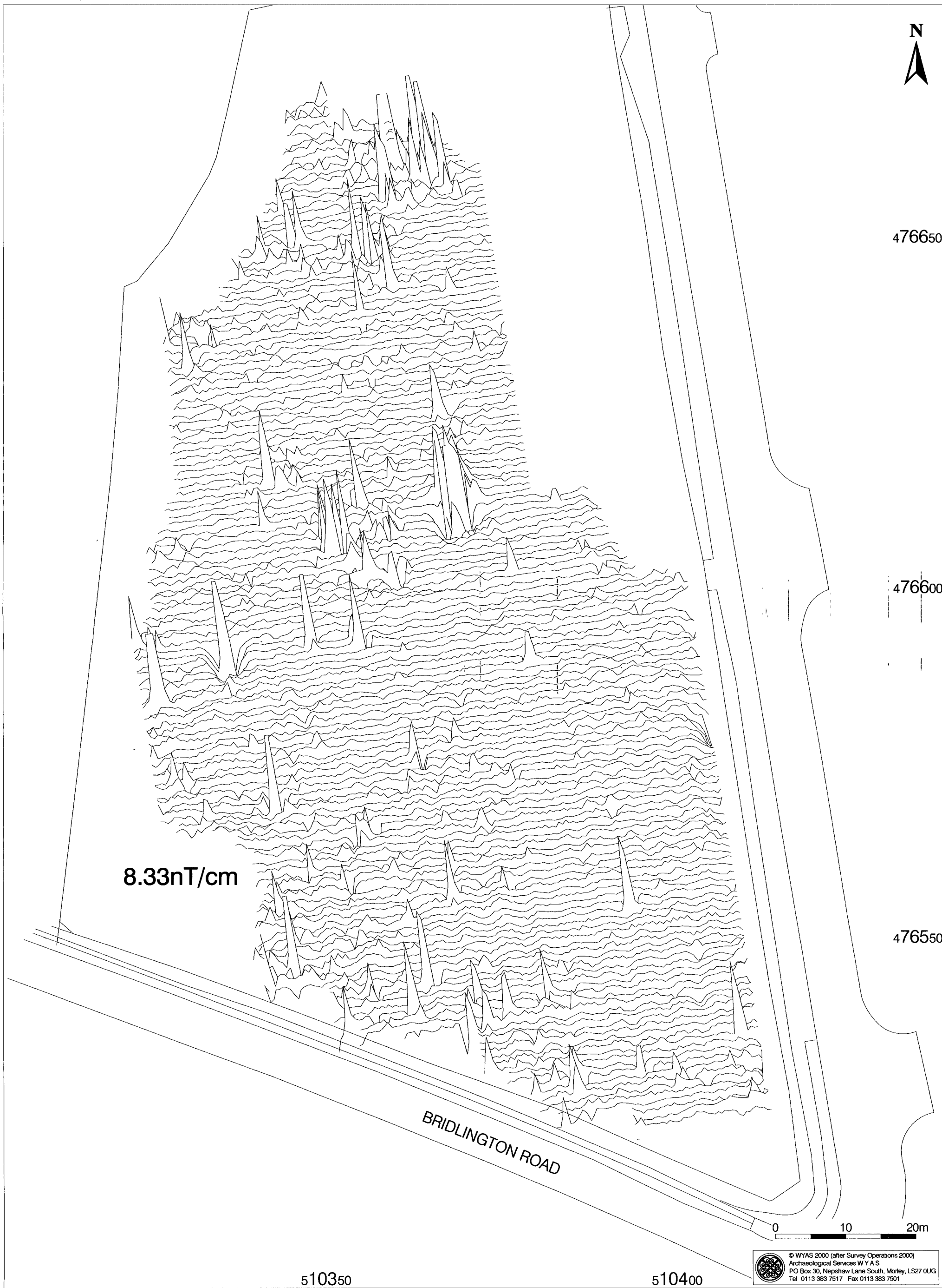
Fig. 4. X-Y trace plot of gradiometer data (1:500)
