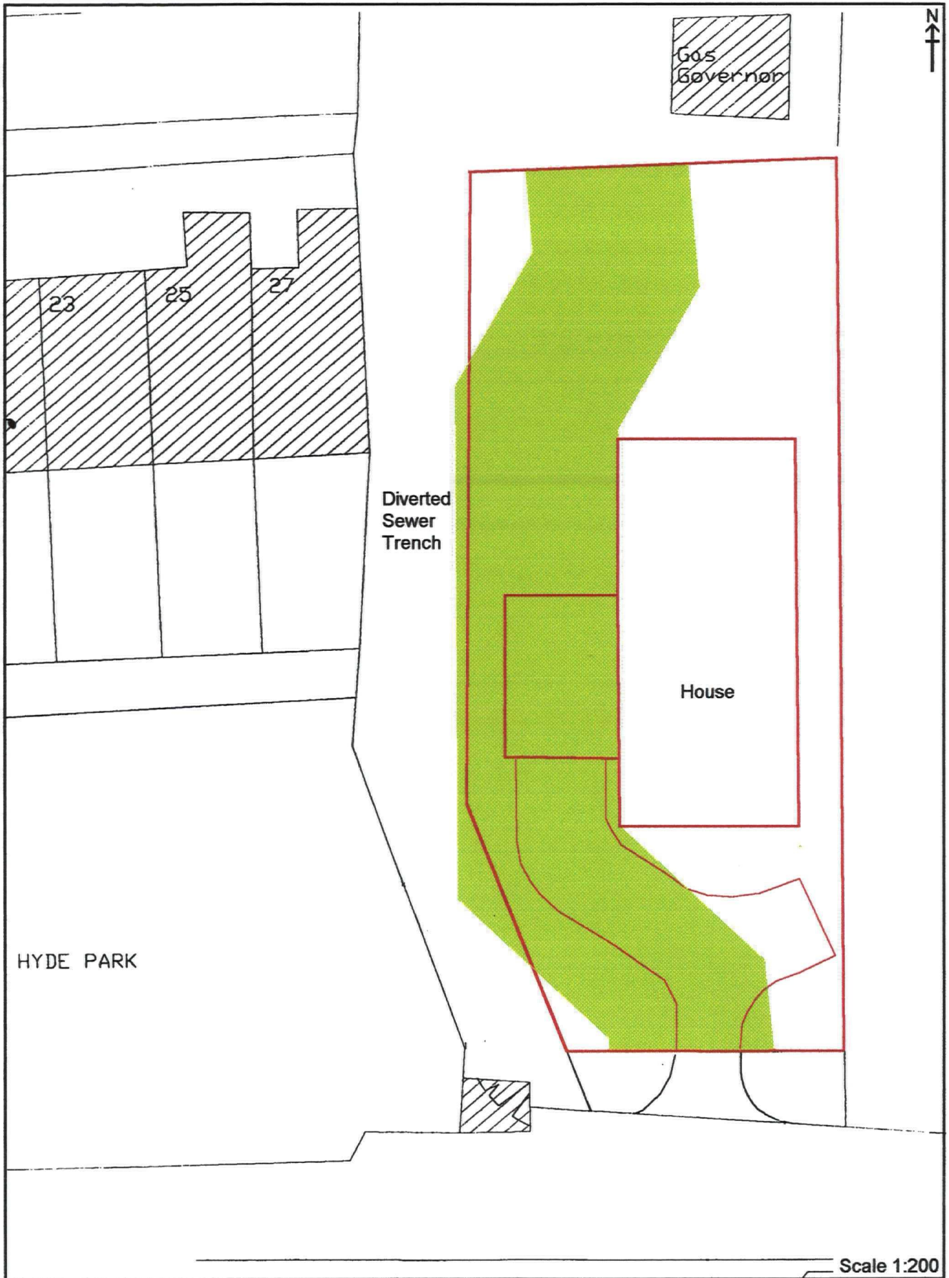
Figure 2. Plan of Sewer Trench and New Development.
