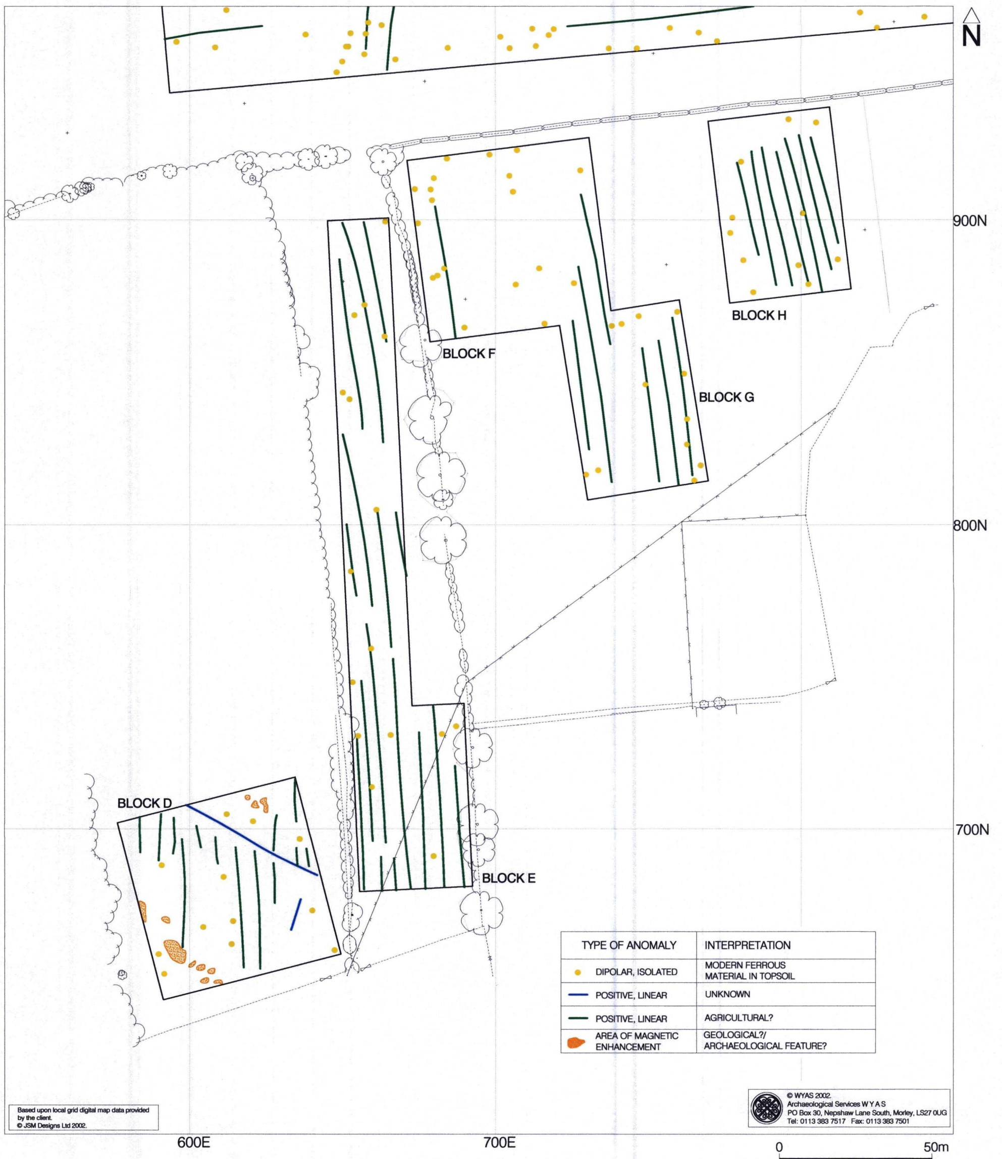
Fig. 8. Interpretation of gradiometer data; Blocks D, E, F, G and H
