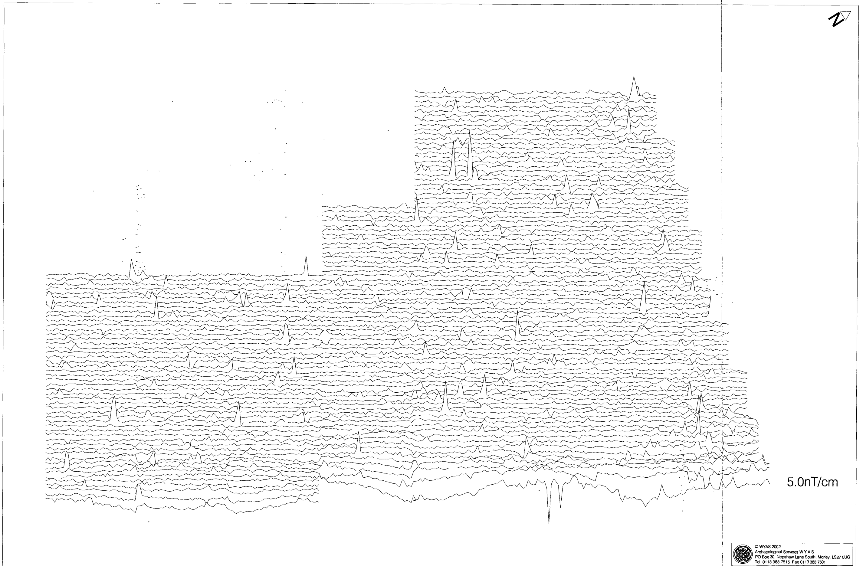
Fig. 30. X-Y trace plot of gradiometer data; Blocks B and C
