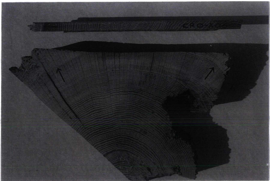
Fig 2. Cross-section of a rafter showing the presence of sapwood rings in the corners; the arrow is pointing to the heartwood/sapwood boundary (H/S). Also a core with sapwood; again the arrow is pointing to the H/S. The core is about the size of a pencil.
