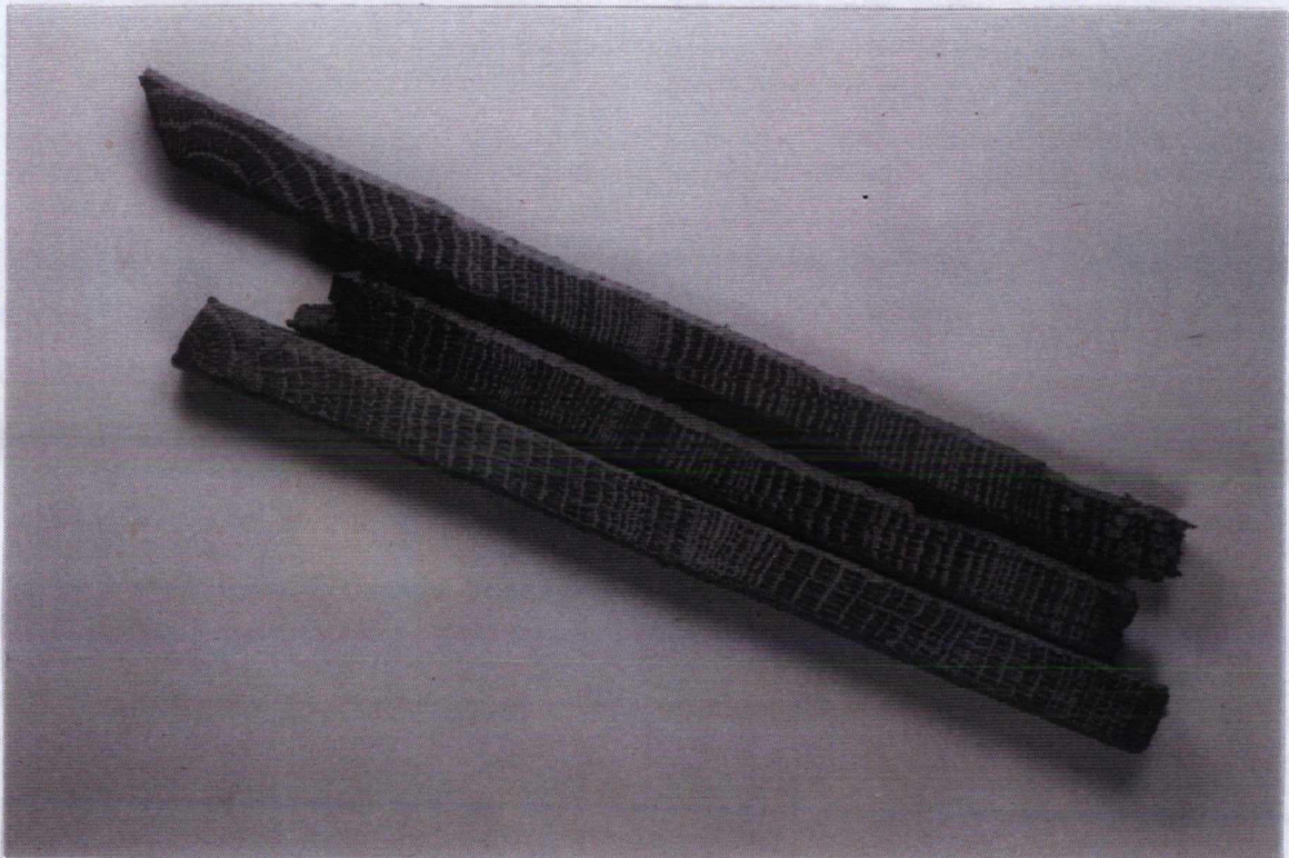
Fig 4. Three cores from timbers in a building. They come from trees growing at the same time. Notice that, although the sequences of widths look similar, they are not identical. This is typical.
