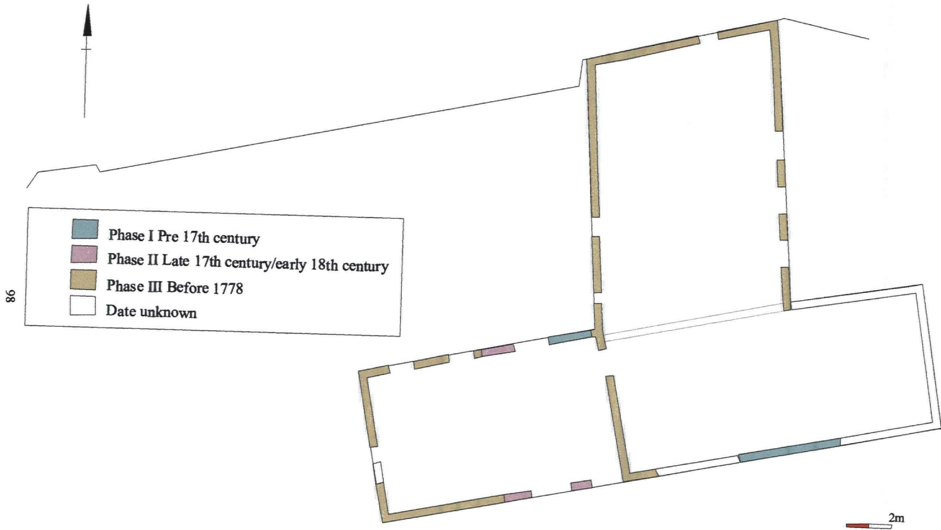
Figure 27, Sketch plan showing phasing of ground plan of Old Sail Loft Do not scale from this drawing
