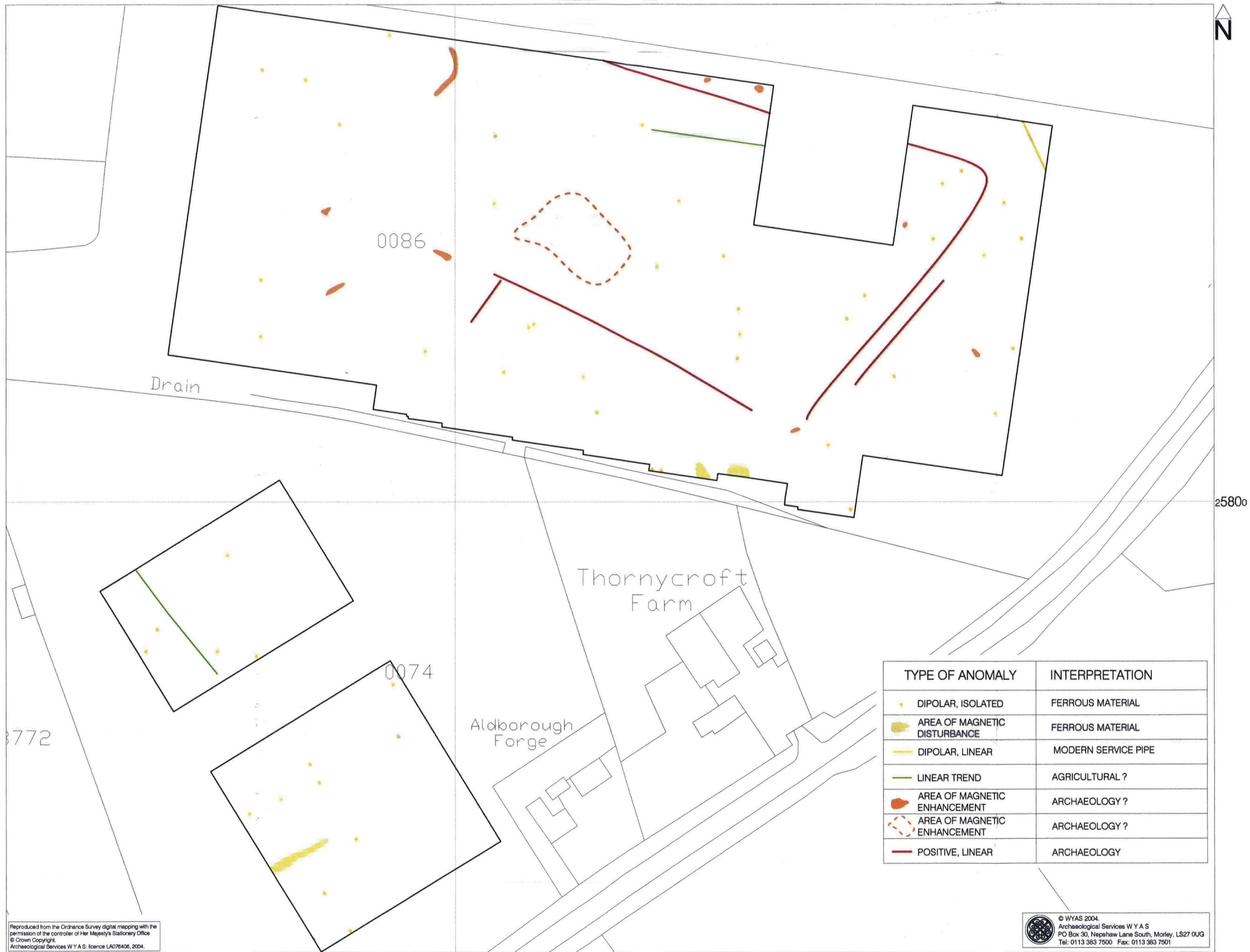
Fig. 4. Interpretation of gradiometer data
