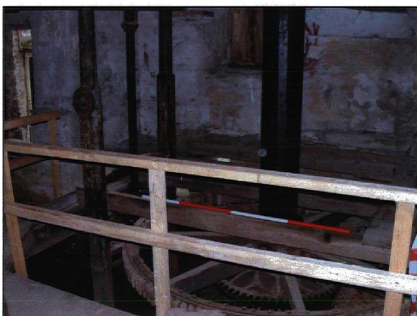
Plate 17. Mill gearing; main shaft, great spur wheel and iron columns with date plate, note also curved recess in wall behind, looking northeast. Scale of 2m.
