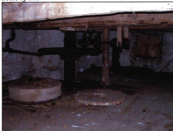
Plate 21. Machinery on the first floor, (stone floor); one set of stones and one lower millstone in situ, main shaft with crown wheel and subsidiary drive, looking southeast.
