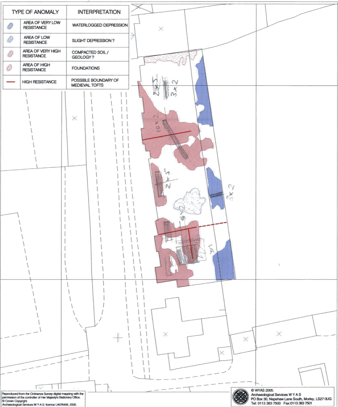
Fig. 6. Interpretation of earth resistance data
