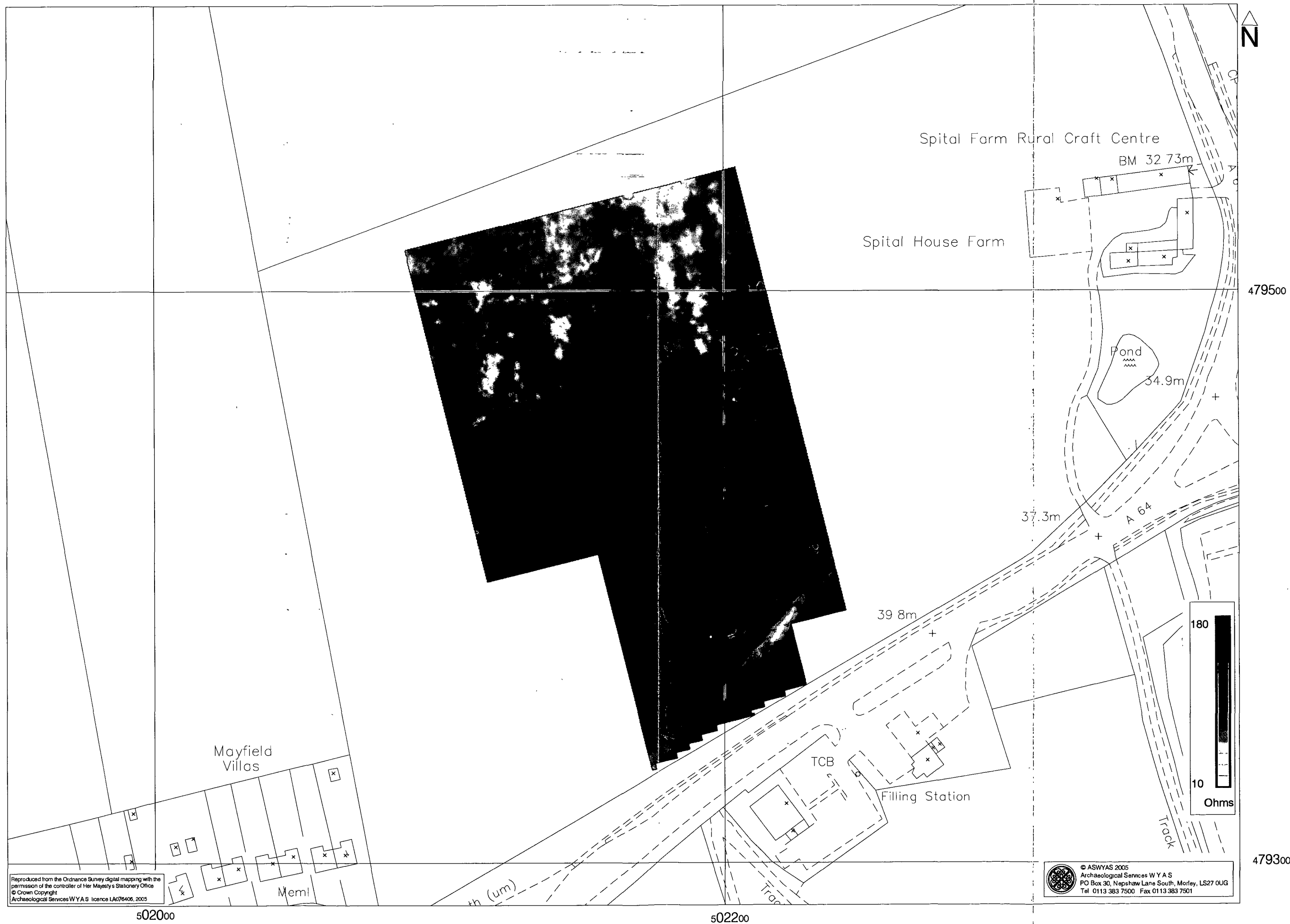
Fig. 9. Plot showing greyscale earth resistance data
