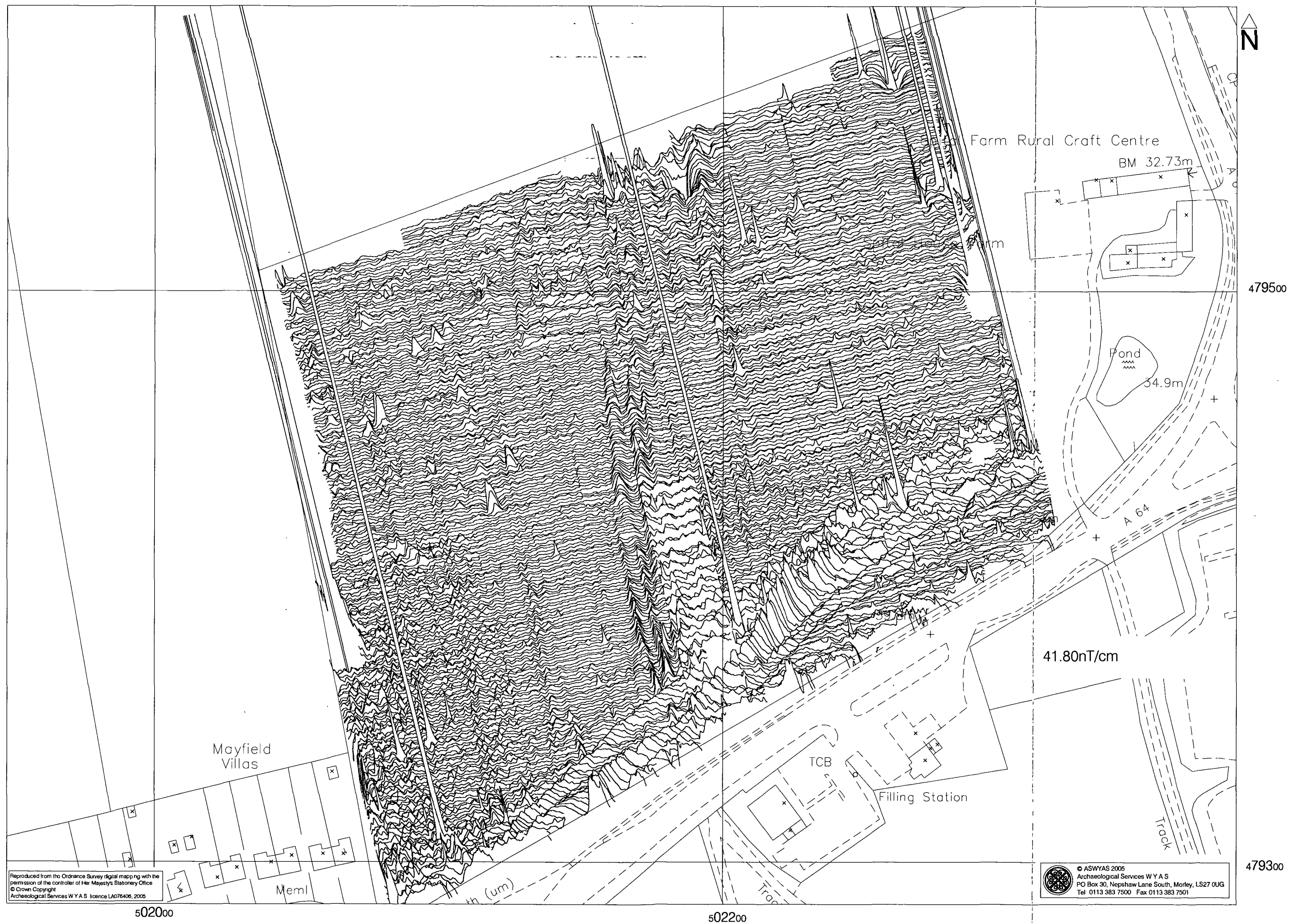
Fig. 7. XY trace plot of magnetometer data
