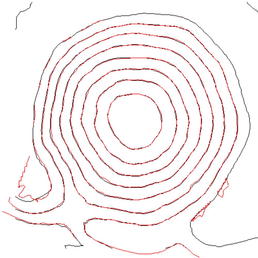
Fig 5. Contour comparison between 1968 and “adjusted” 2001 surveys at 5-metre intervals. Note close correspondence between models except around base.
