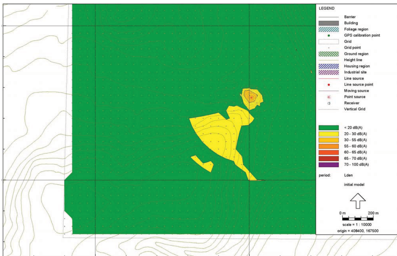
409000 410000 Industrial Noise -ISO 9613.1/2, WHS -landform profile of WHS -initial model [D:\silbury2\] , Predictor Type 7810 V5.04
