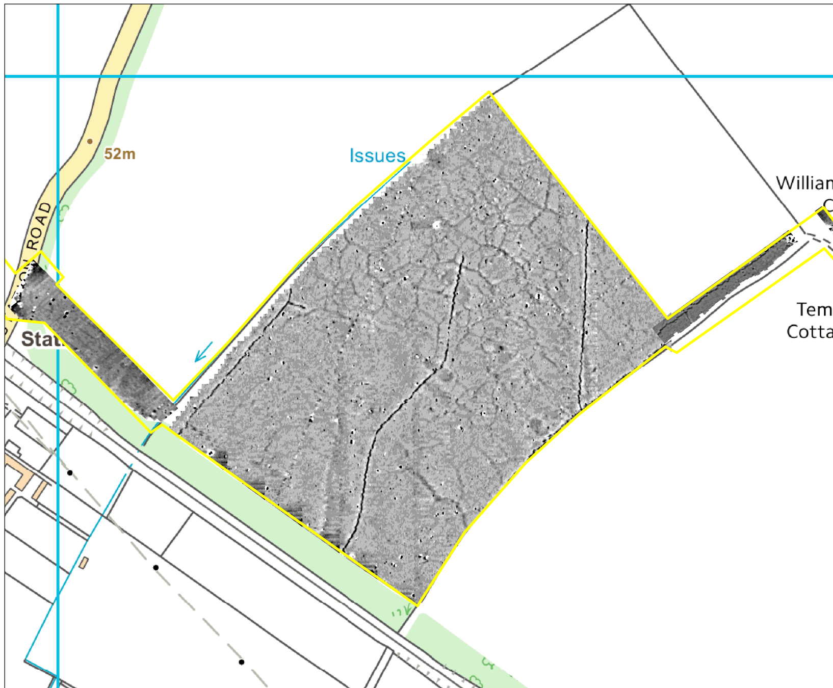
Figure 6: Processed Geophysical Data, Section 1
