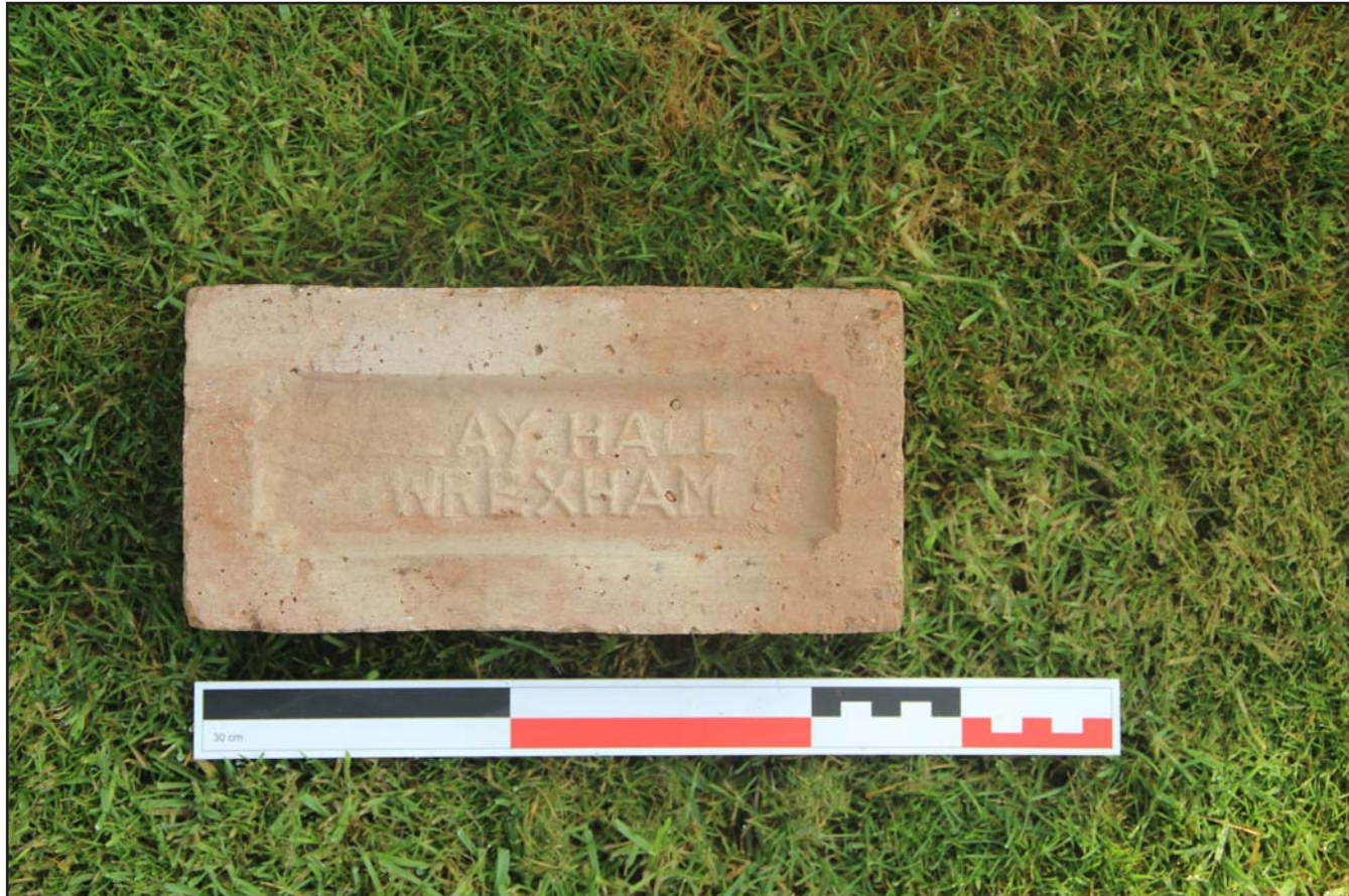
Plate 05: Example of brick used in wall construction, stamped "LLAY HALL WREXHAM" - scale 0.3m
