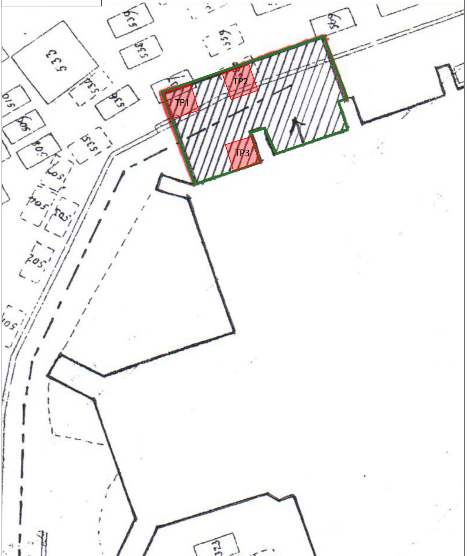
Figure 03: Location of Test Pits 1-3 (TP 1-3) at St Oswald's Church, Malpas overlain on the 1884 Graveyard Plan. Scale 1:100 at A4.
