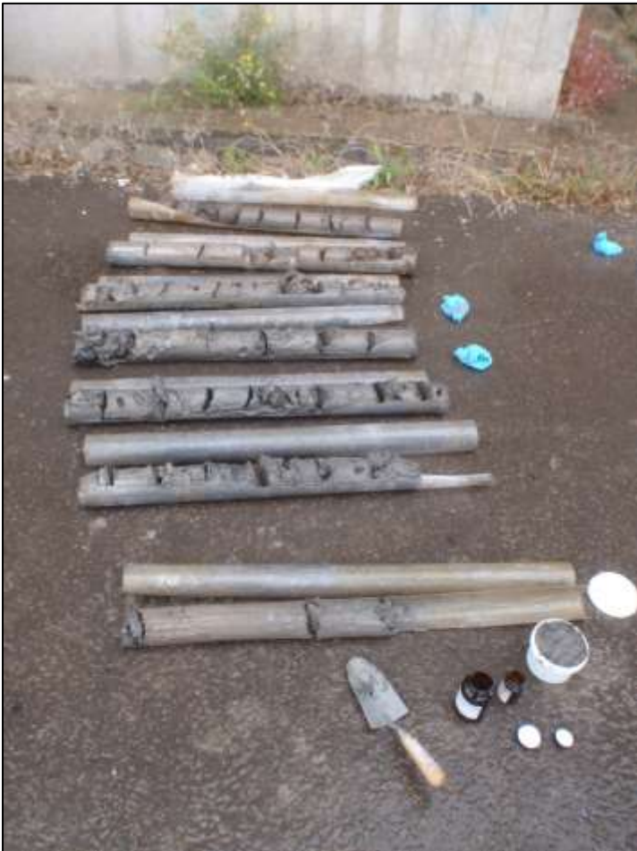
Plate 10. Borehole SBH 01 cores showing alluvial clay, all 1m lengths.
