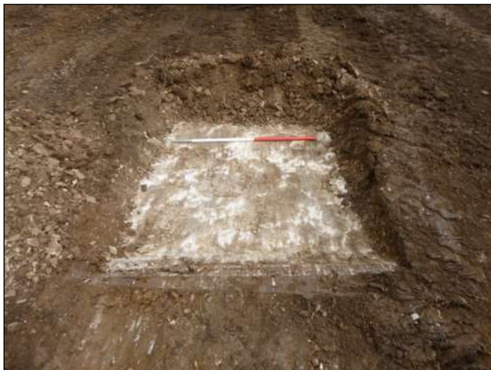
Plate 4: Example of geotechnical trial pit showing depth of supsoil above bedrock
