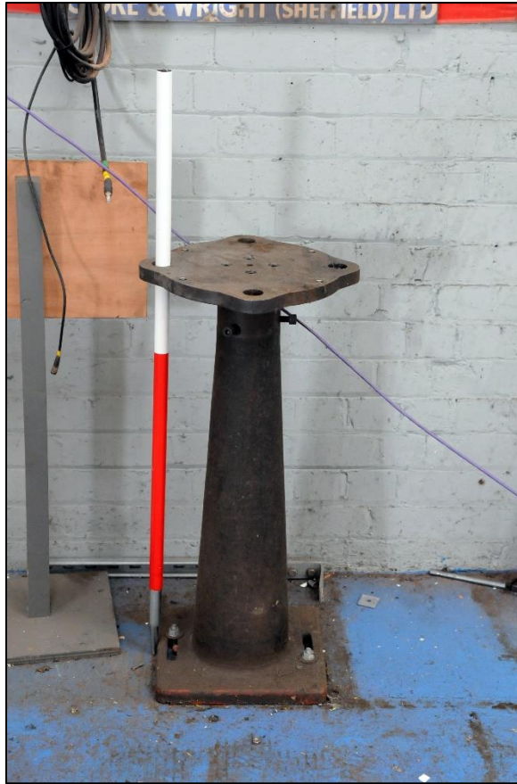
Plate 27: Detail of heavy vice stand, western range of Building 4 (image 0025).
