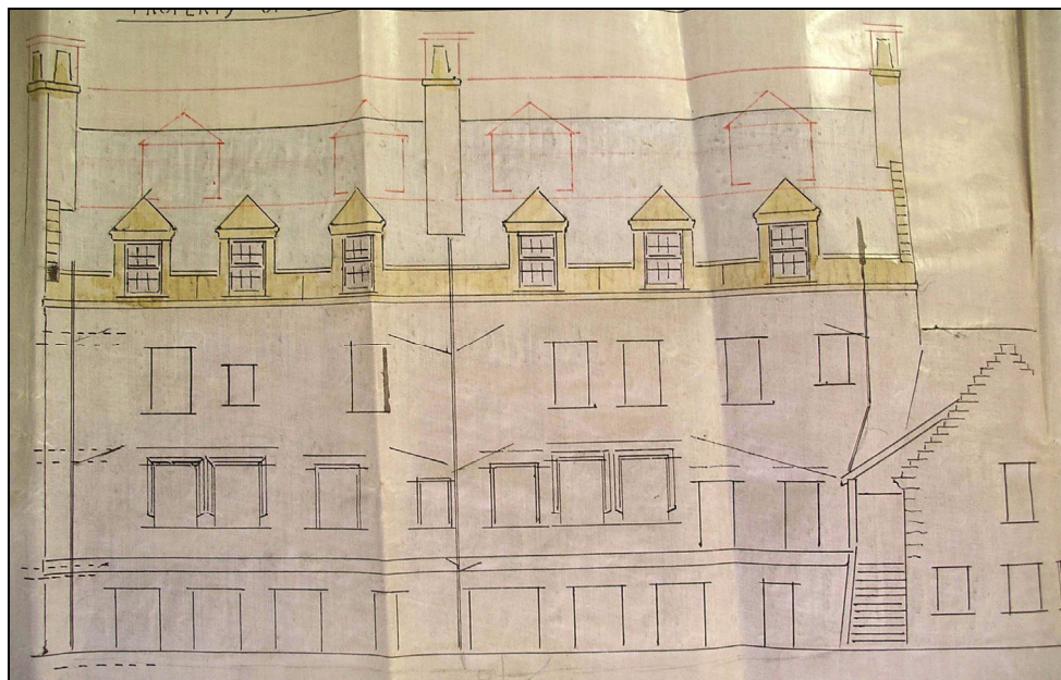
Figure 2-8: Thomas Ross 1916 restoration: Front elevation. The former top floor in red outline, new work in yellow.
