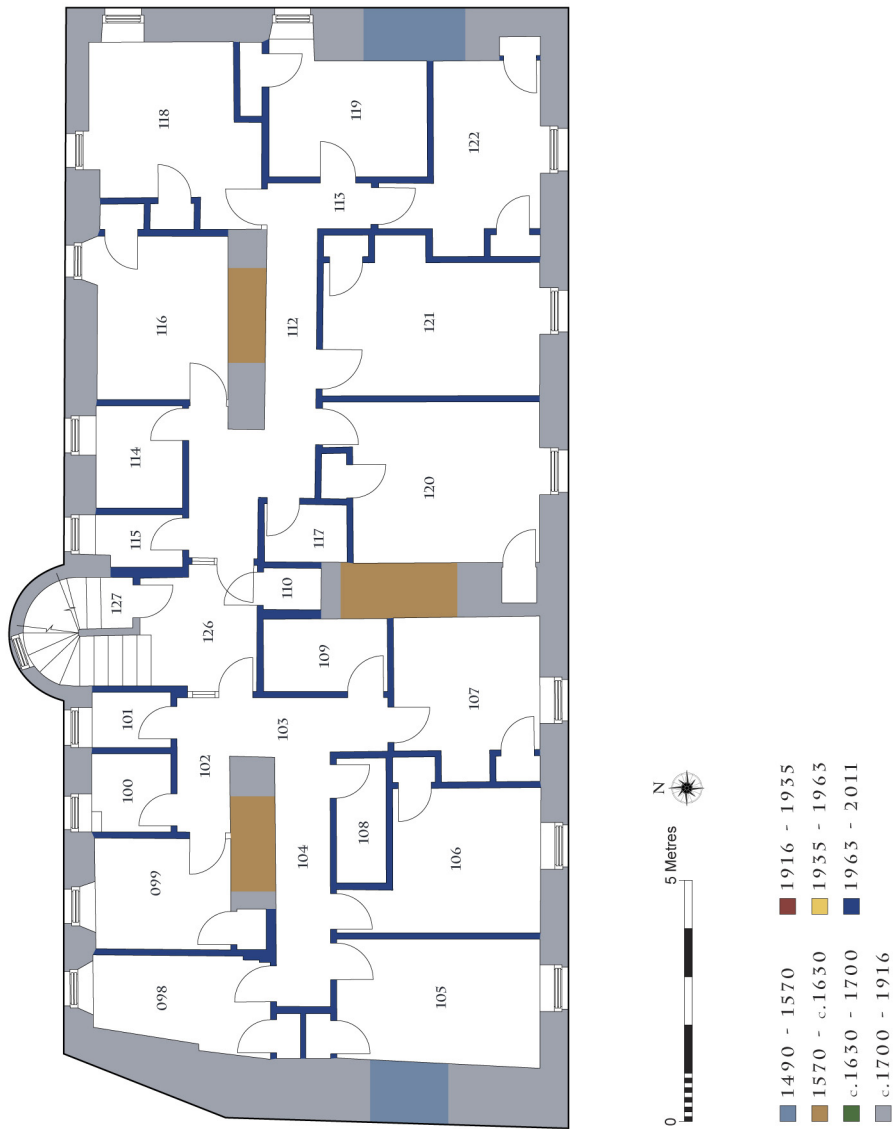
Figure 3-4: Periodised Third Floor plan with Component Numbers
