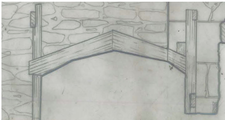
Fig. 132-31 View from east showing ceiling-rib 085 and strips 088 and 092 of northern dormer.
