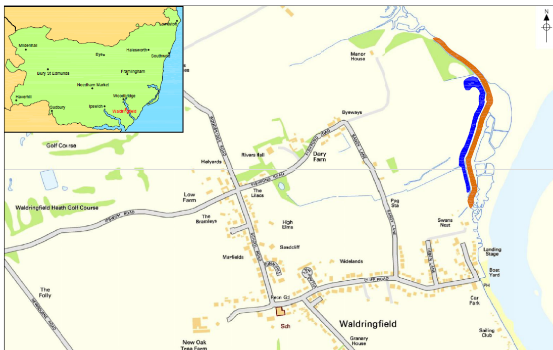
Fig 1. Site location showing new dyke (blue) and strengthened section of flood bank (orange).
