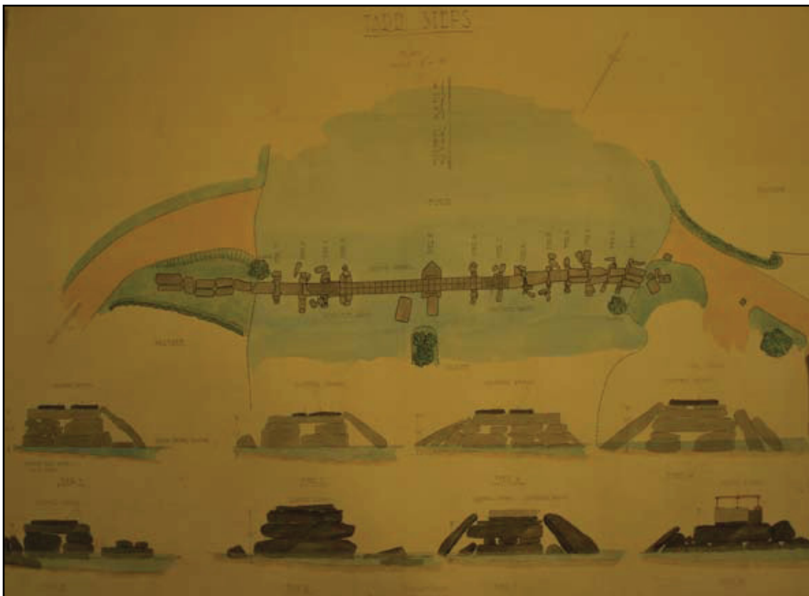
Fig 27 (above) Elevation drawings of piers (detail) which show the structure of Tarr Steps before it was swept away in the 1952 floods (SRO A\BHN/3)
