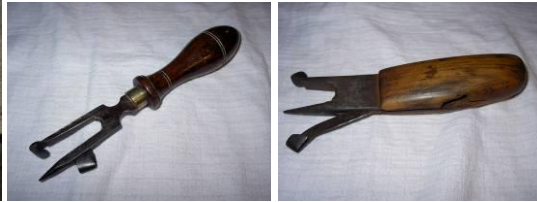
Merchants mark in the East Stables. C19th and C20th race knives and circle scribes.
