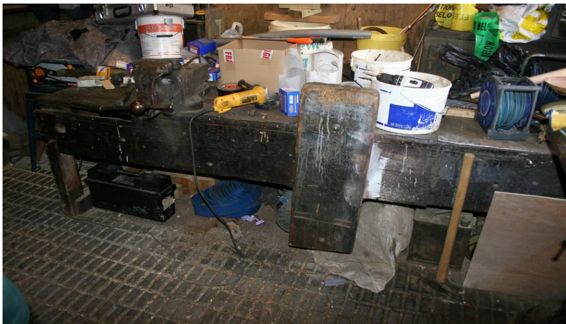
Workbench with engineers' and saddler's vice.
