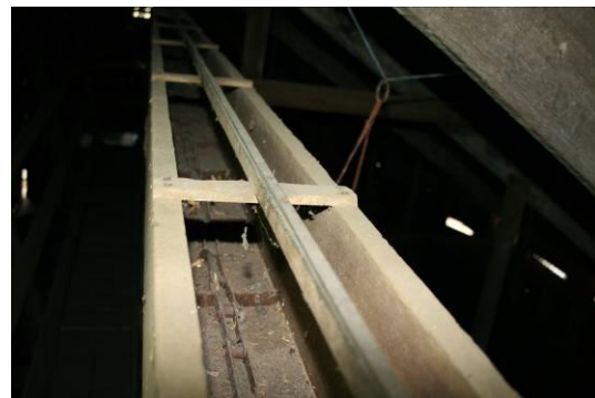
Detail of the chain drive in the upper channel.
