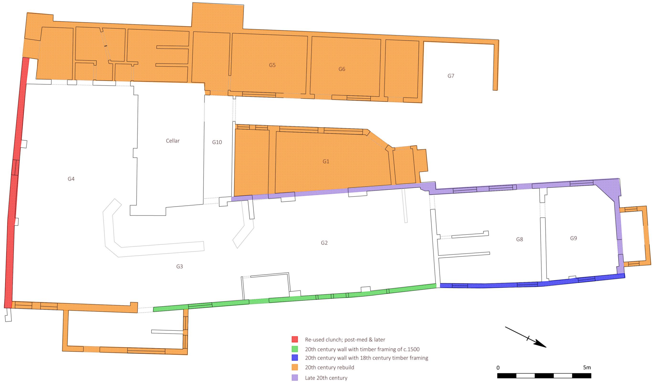
Figure 24: Phase plan (scale 1:100)
