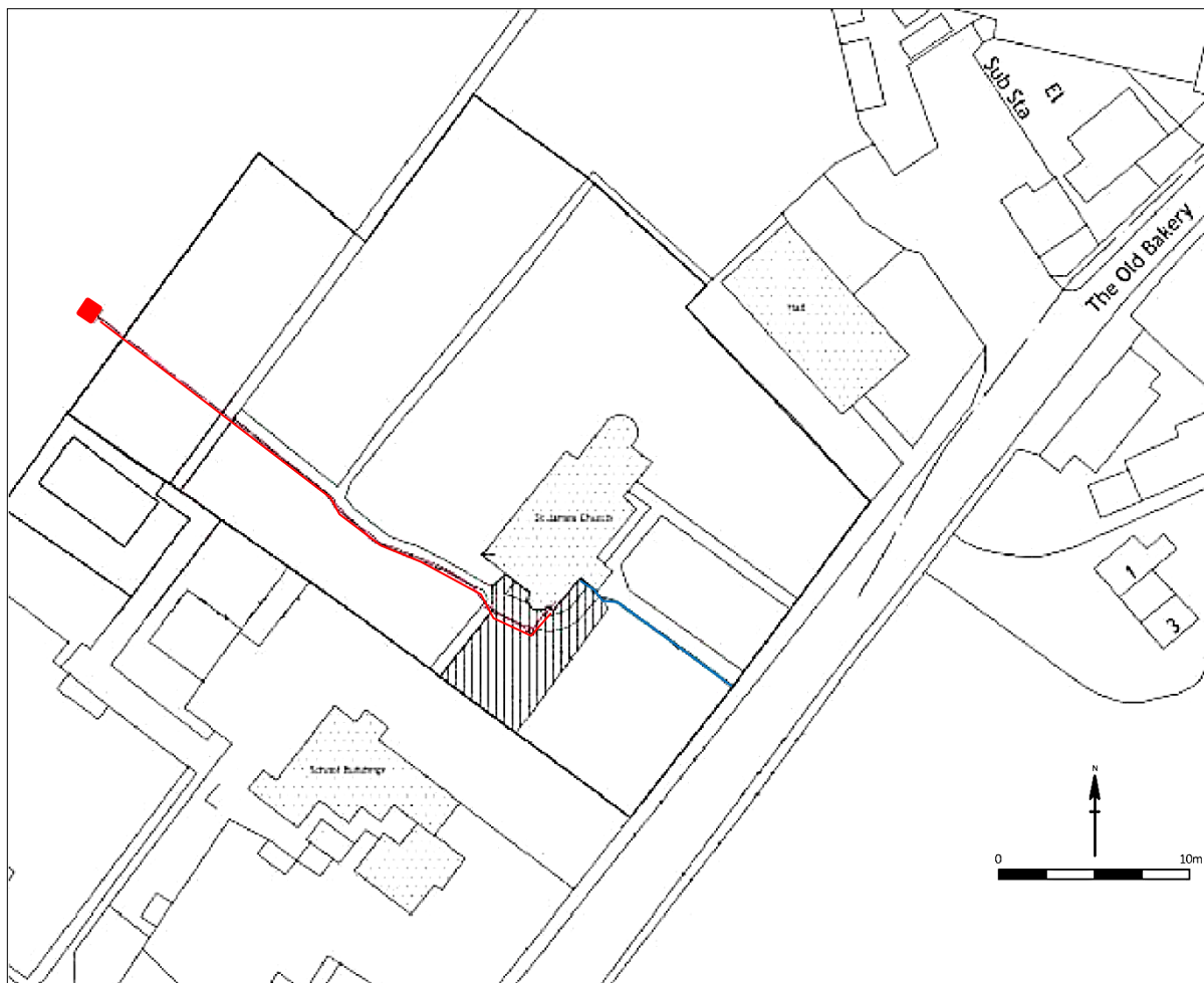
Figure 3: Proposed services route (red shows drainage, blue shows water supply) (scale as shown)
