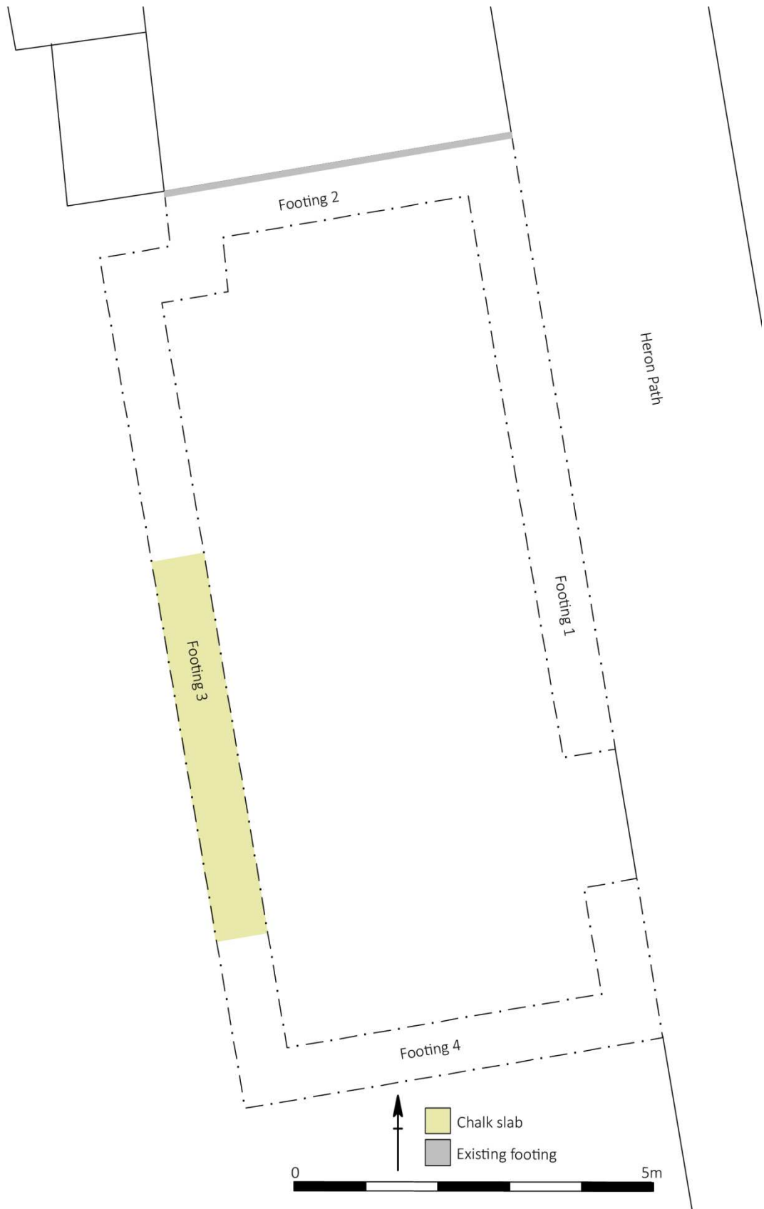
Figure 7: Plan of footing trenches (scale 1:75)
