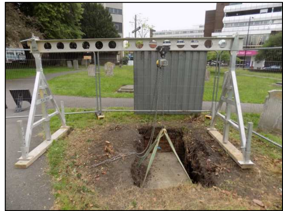
Plate 4: Mechanism used to lift the ledger
