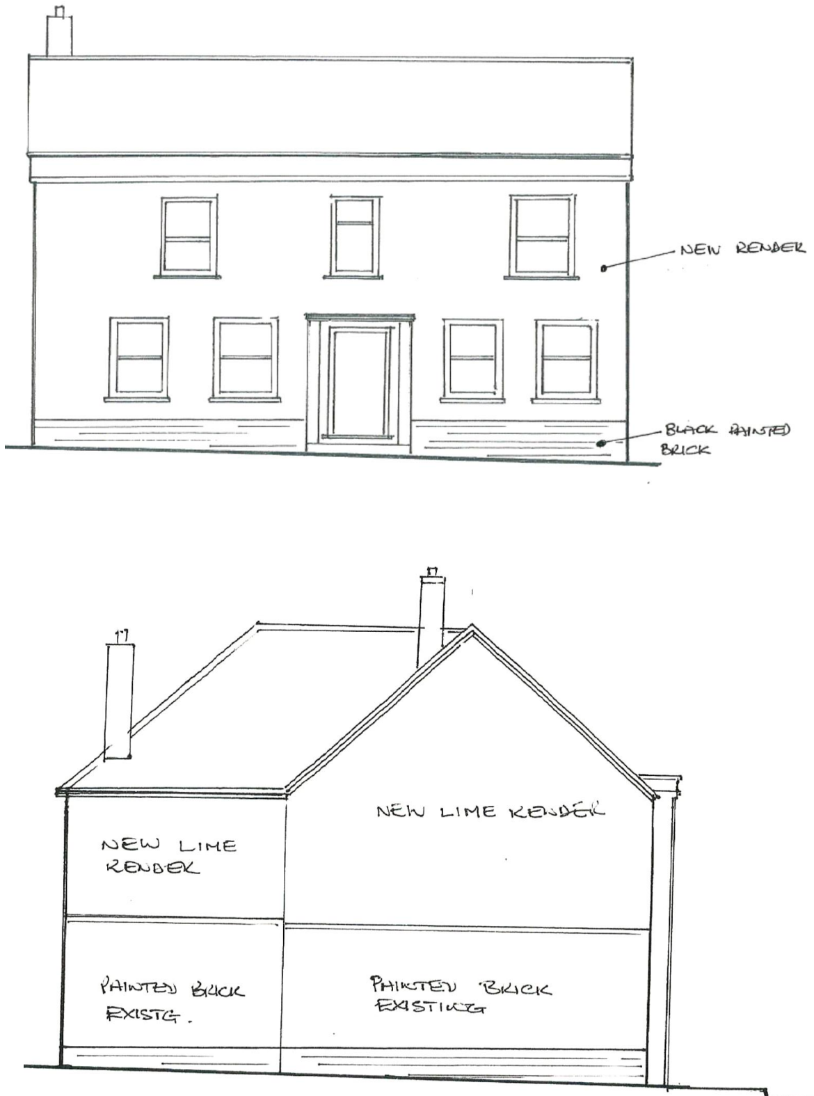
Figure 3: Remedial works– front elevation (top) and flank (east) elevation (bottom) (not to scale)
