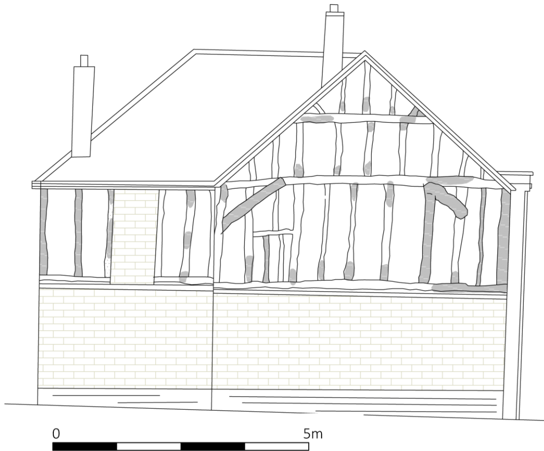
Figure 12: East elevation showing decayed timbers (scale 1:75)
