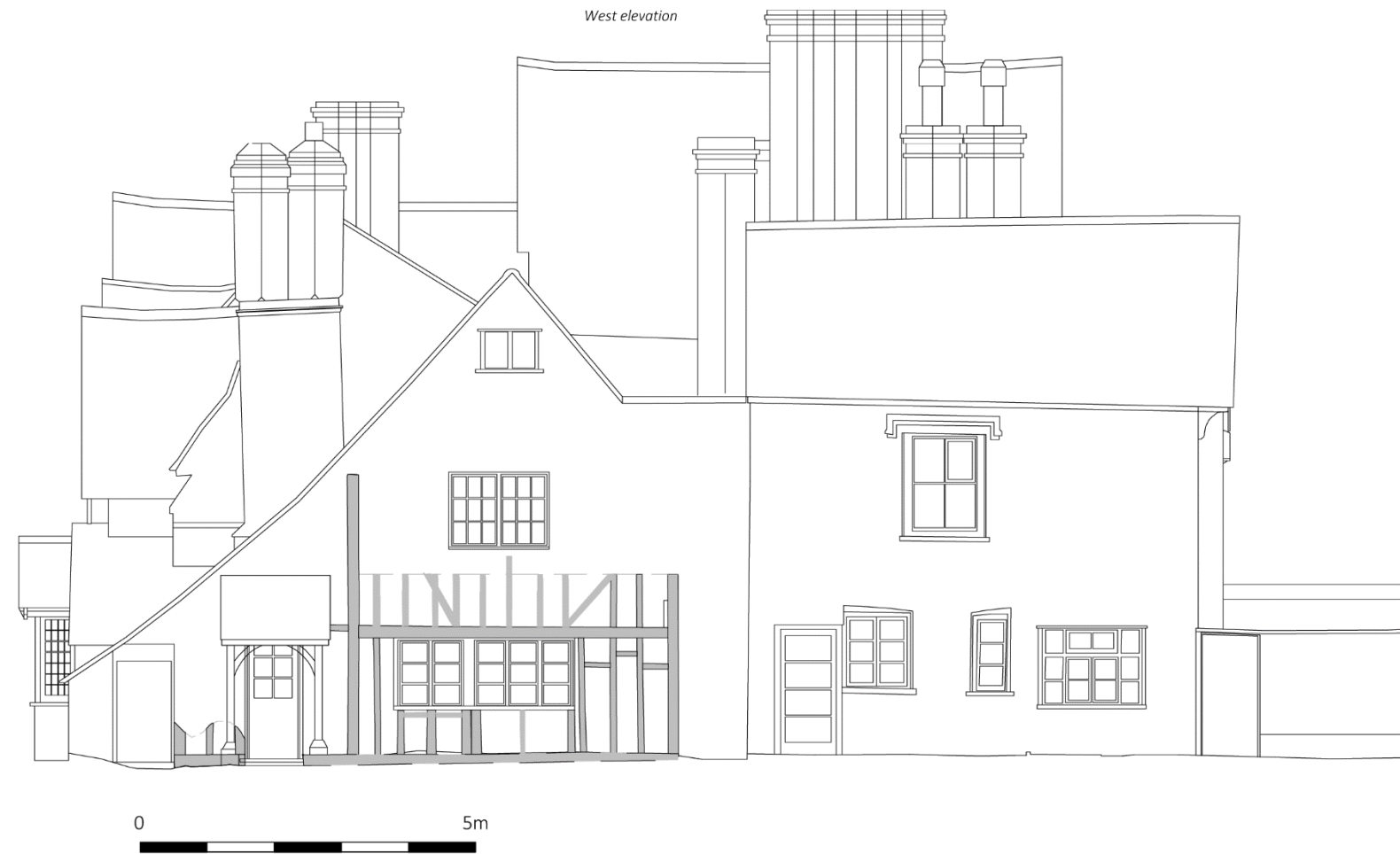
Figure 8: West elevation showing the timberwork exposed during the building works (scale 1:100)
