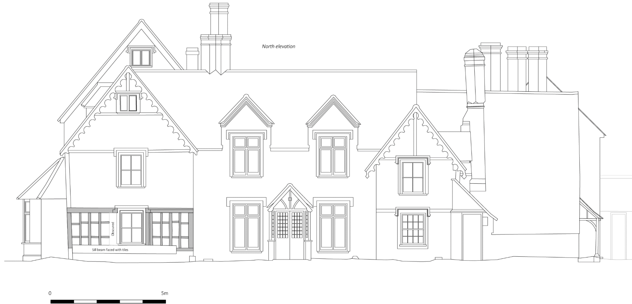
Figure 5: North elevation showing the timberwork exposed during the building works (scale 1:100)
