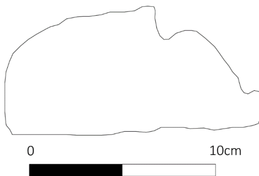
Figure 3: Mid-19 th century moulded brick section (scale 1:2)
