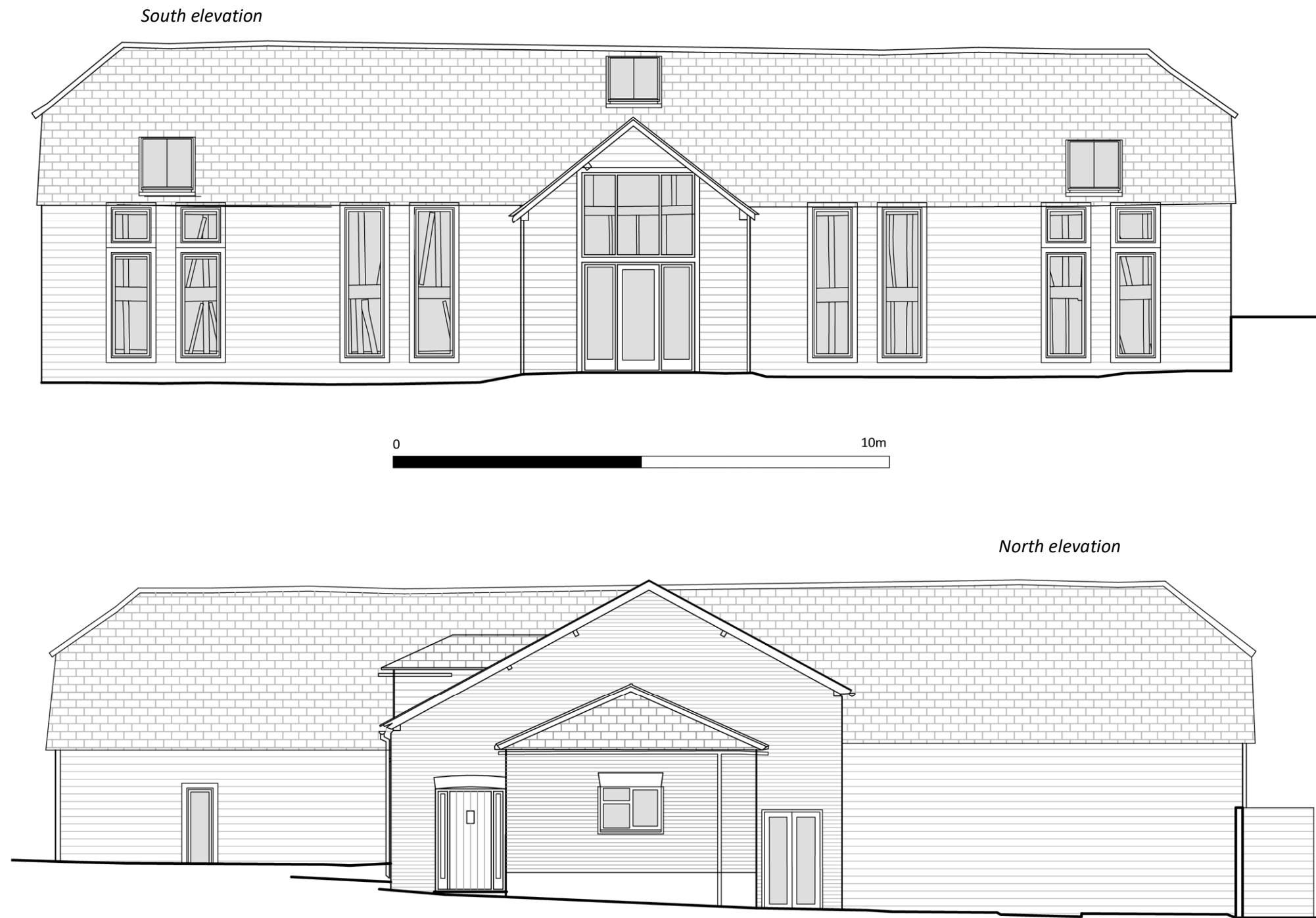
Figure 20: Barn 1 proposed south and north elevations (scale 1:100)
