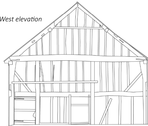
Figure 15: Barn 1, east and west internal elevations (scale 1:100)
