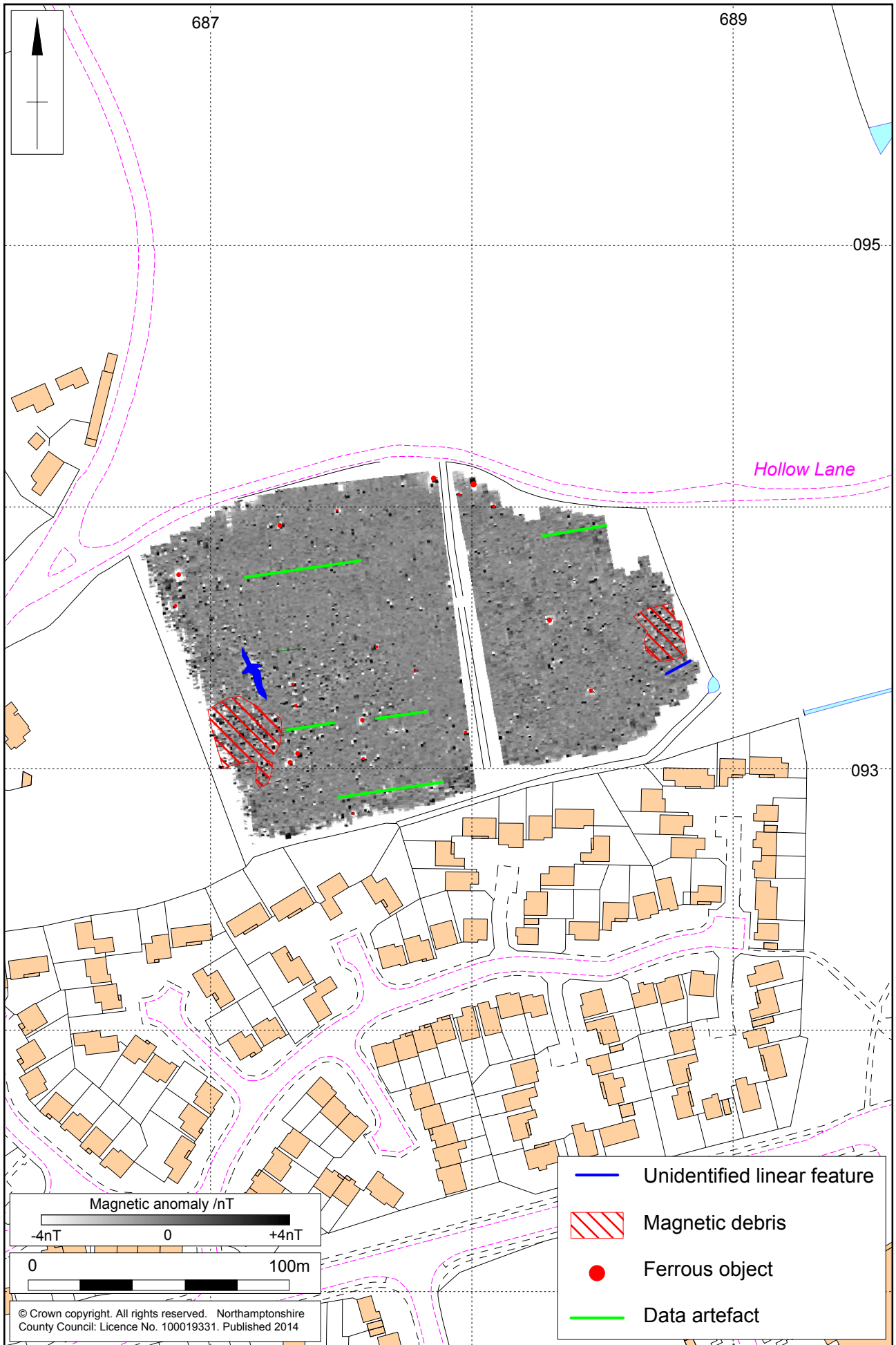
Magnetometer survey interpretation Fig 3
