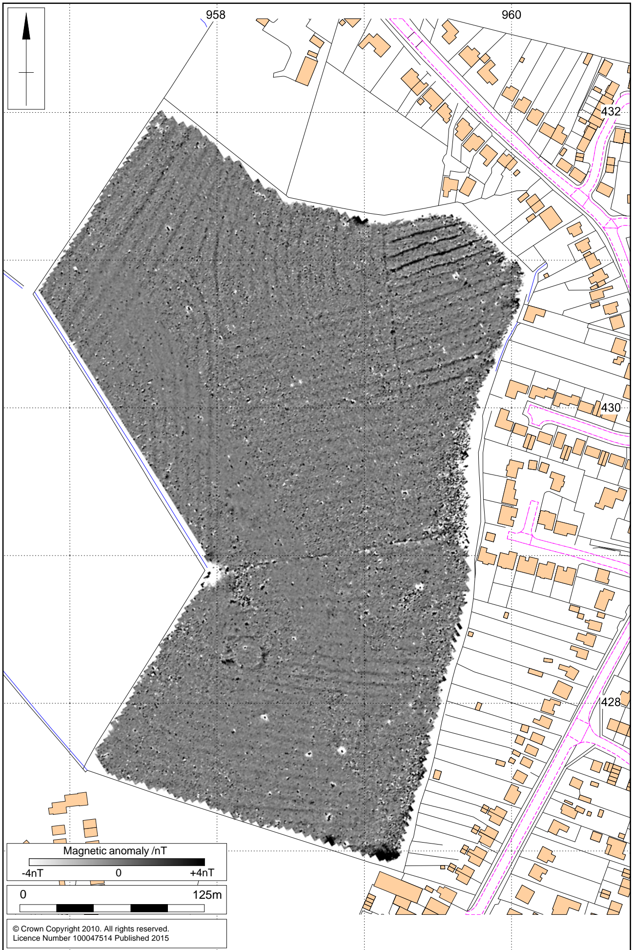
Magnetometer survey results Fig 2
