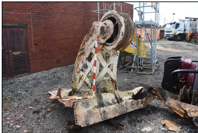
Detail of inner lift roller carriage following detachment Fig 34
