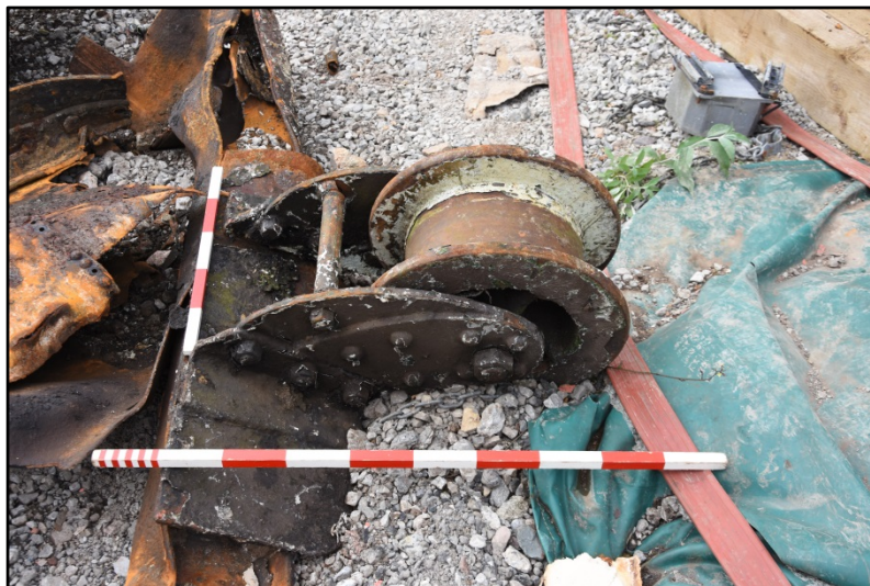
Detail of outer lift roller carriage Fig 35
