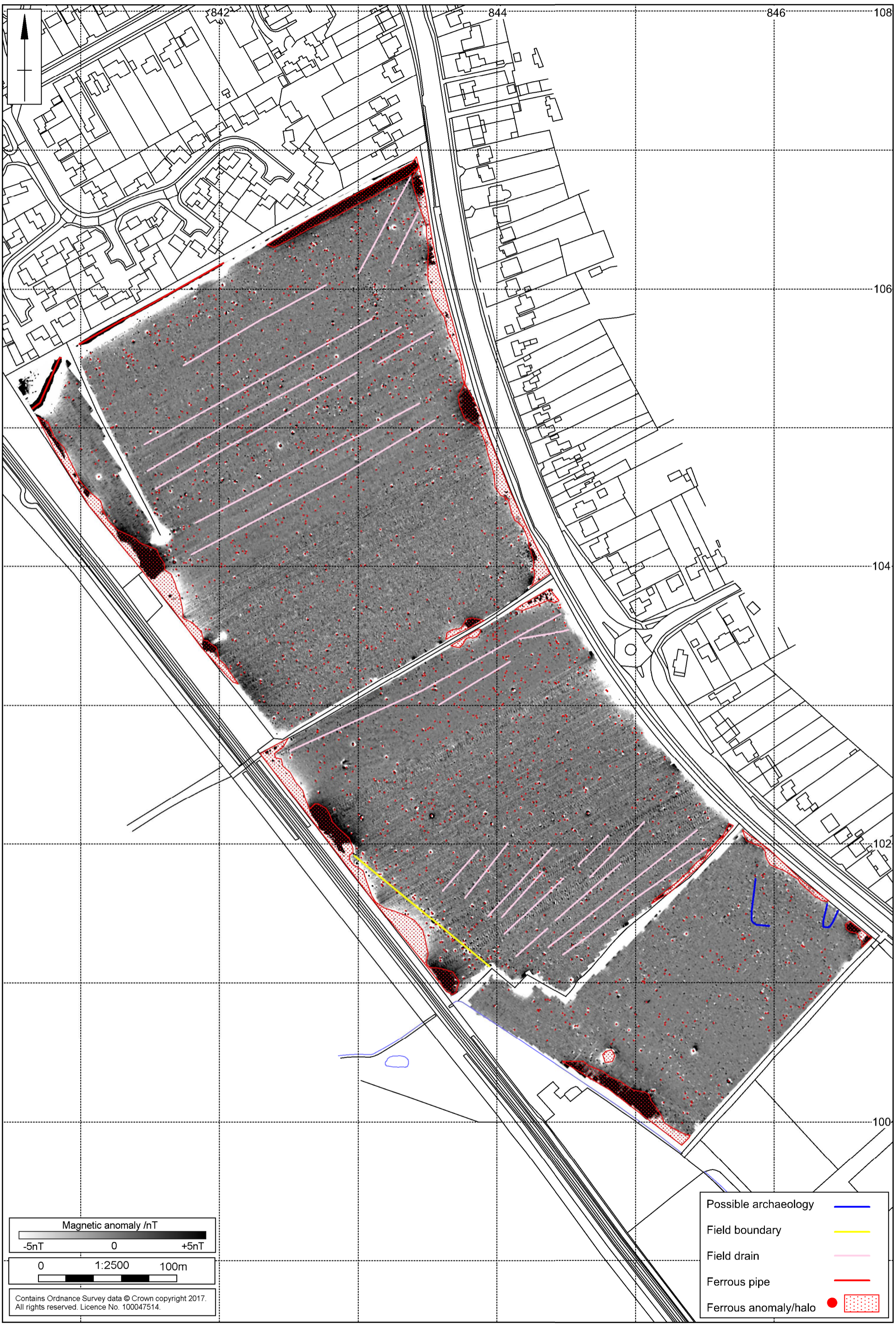
Magnetometer survey interpretation Fig 3
