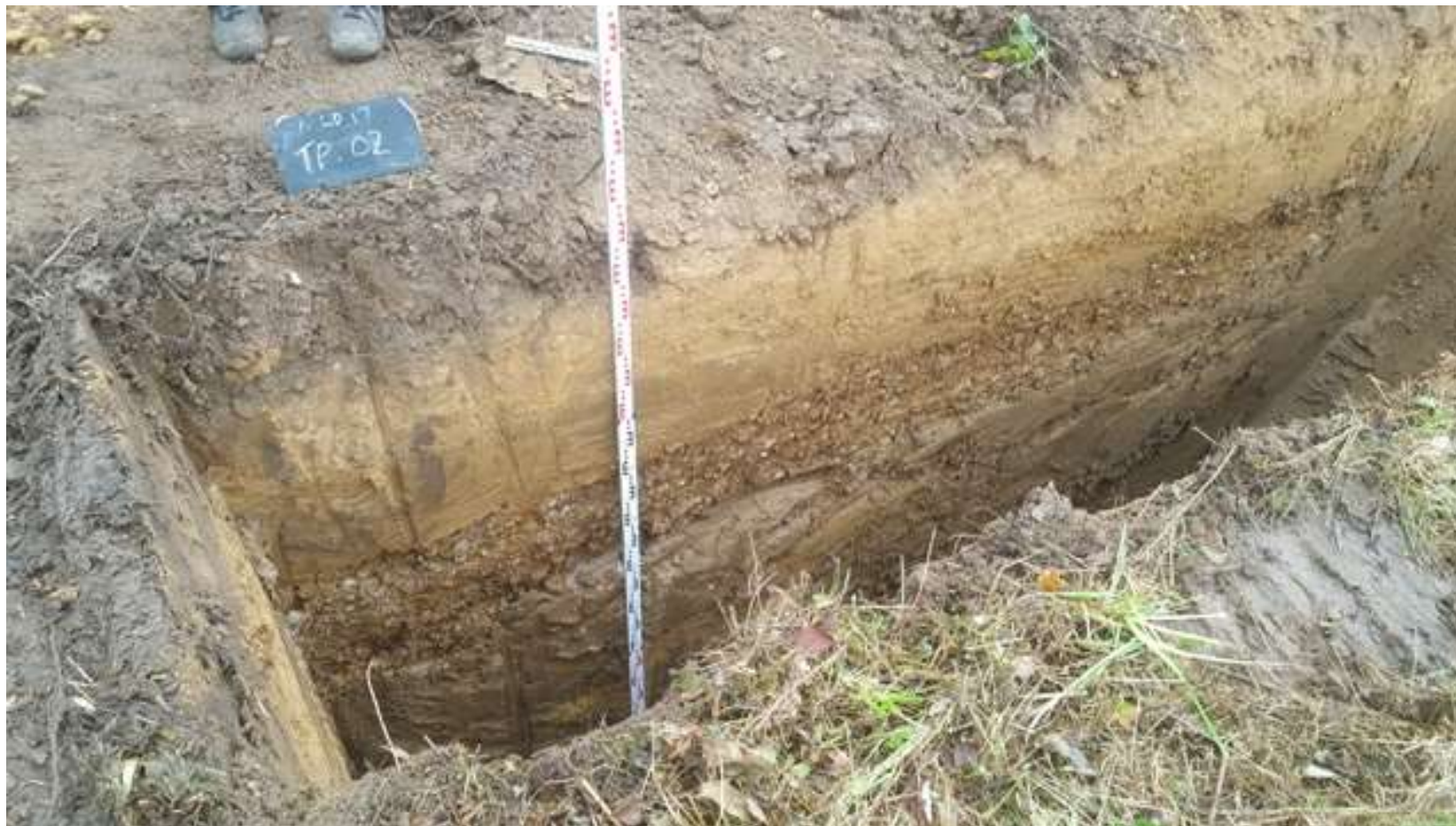
Photo 9: Test pit 2 showing gravel layer in section
