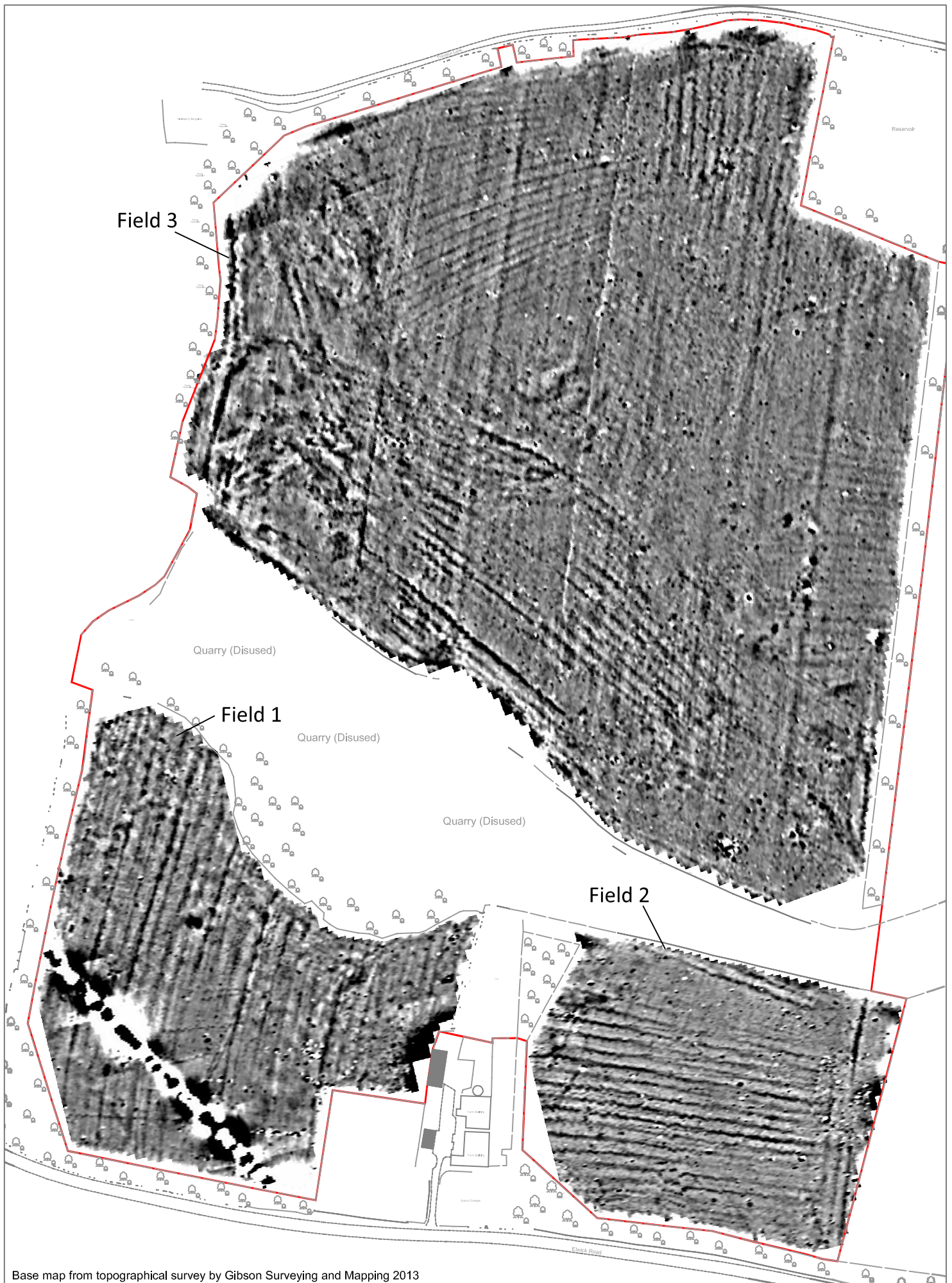
Figure 9: Overall greyscale plot of processed geophysical survey
